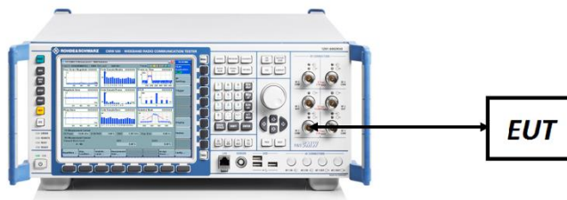
Figure 7-4. ERP/EIRP Measurement Setup
