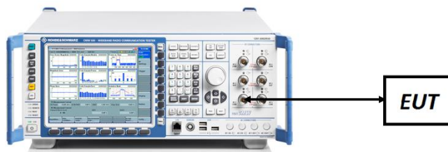
Figure 7-4. Conducted Power Measurement Setup
