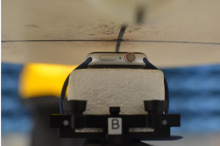
SAR Test Setup Photo 3: Aluminum with Sport Wristband, Front side at 1.0 cm
