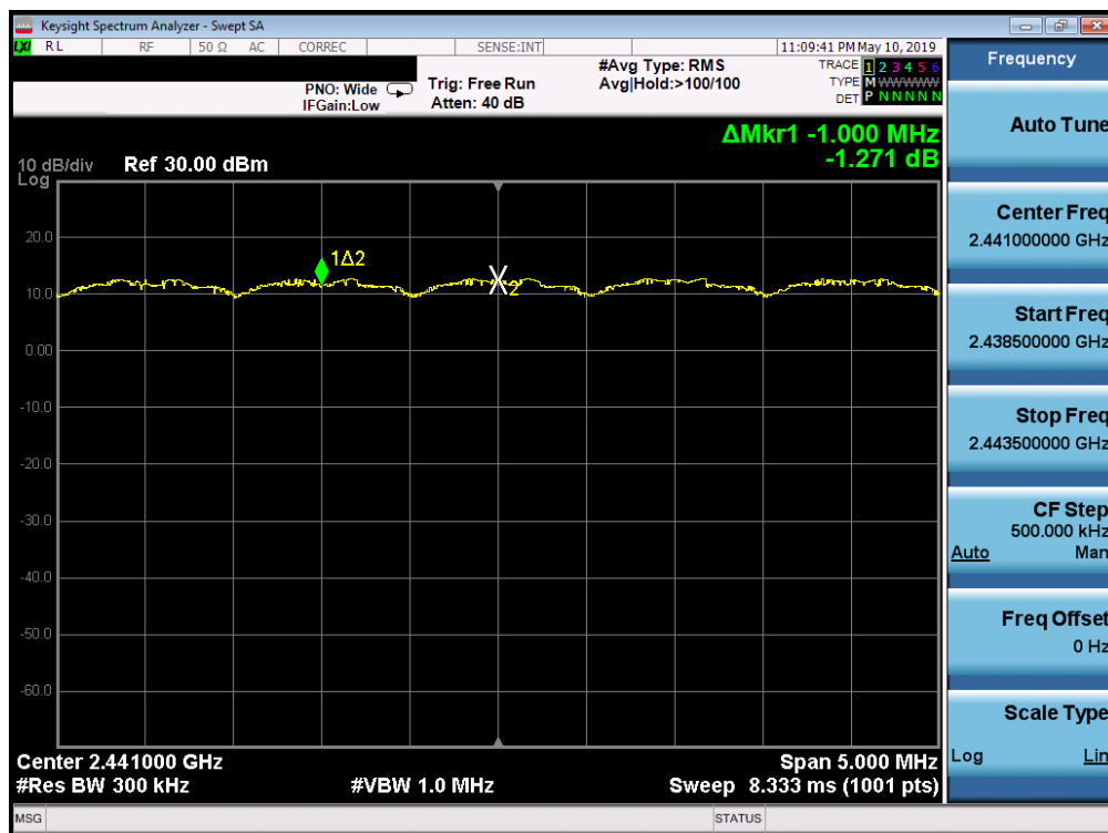
Plot 7-16. Channel Spacing Plot (Bluetooth, 8DPSK, ePA)
