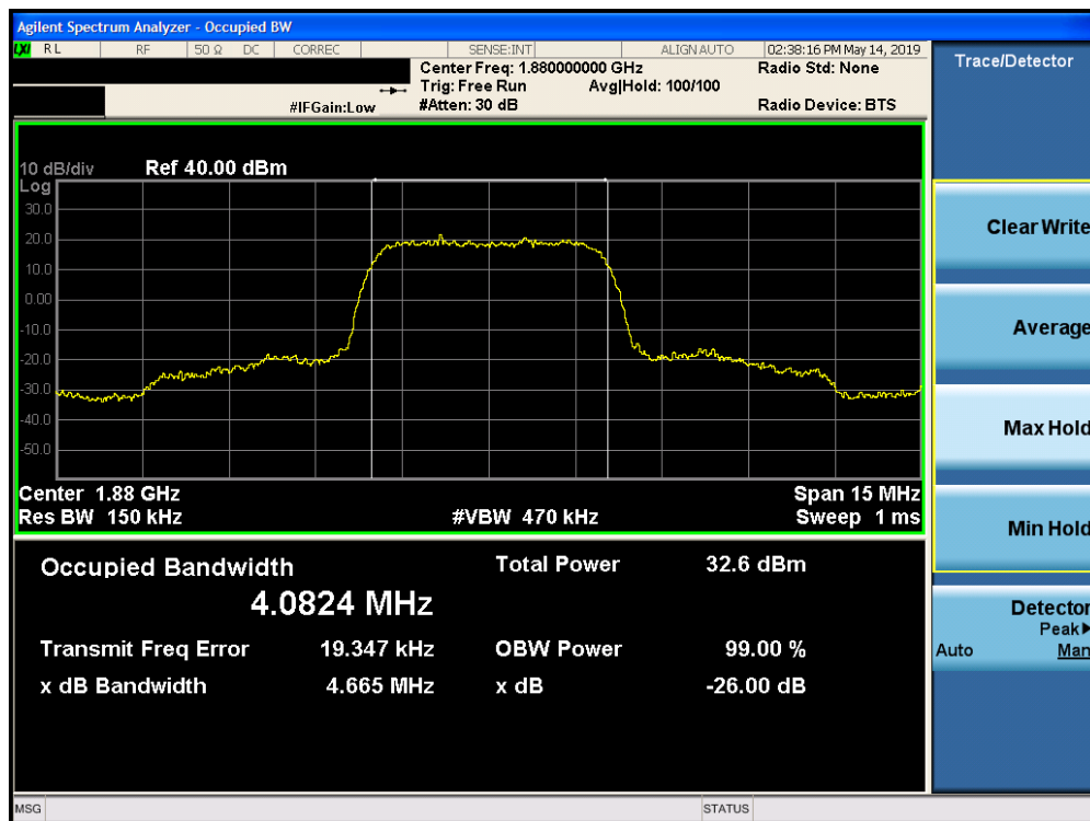
Plot 7-3. Occupied Bandwidth Plot (PCS WCDMA Mode)
