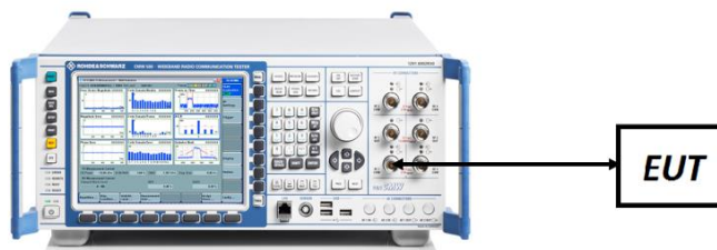
Figure 7-5. ERP/EIRP Measurement Setup
