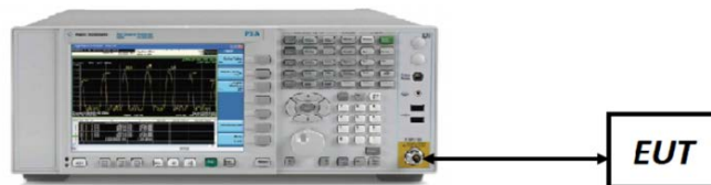
Figure 7-5. Test Instrument & Measurement Setup
