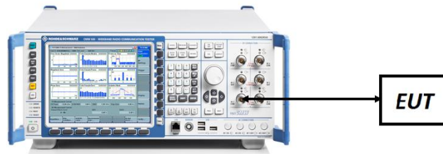
Figure 7-4. Conducted Power Measurement Setup
