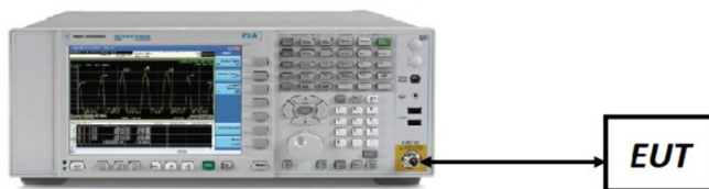
Figure 7-5. Test Instrument & Measurement Setup
