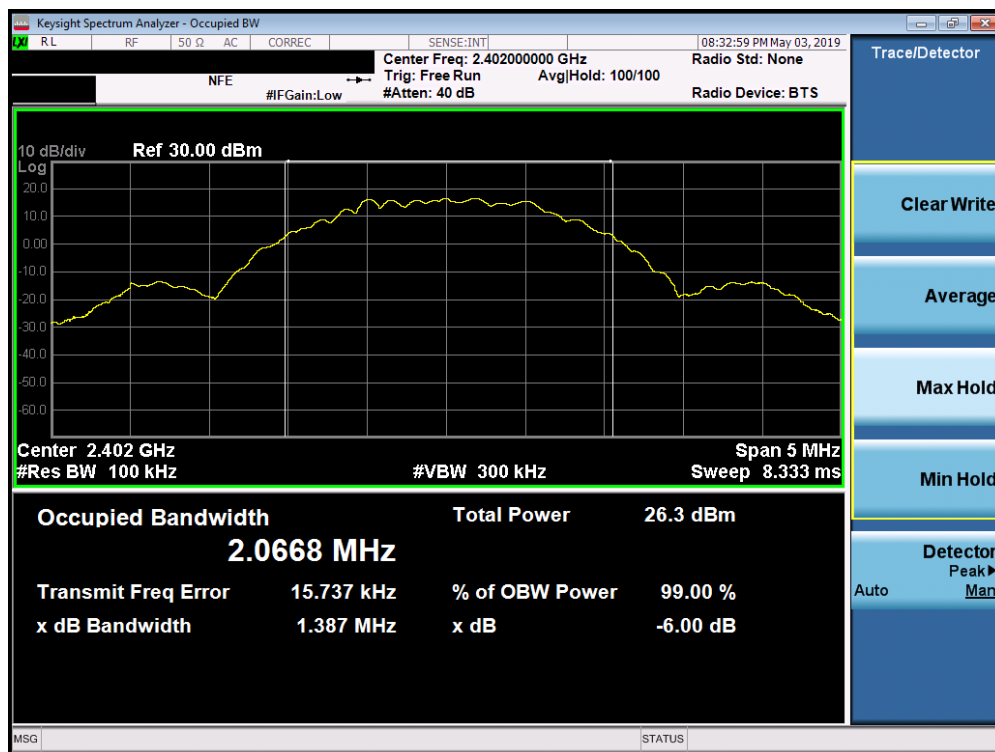
Plot 7-4. 6dB Bandwidth Plot (Bluetooth (LE), 2Mbps ePA – Ch. 0)
