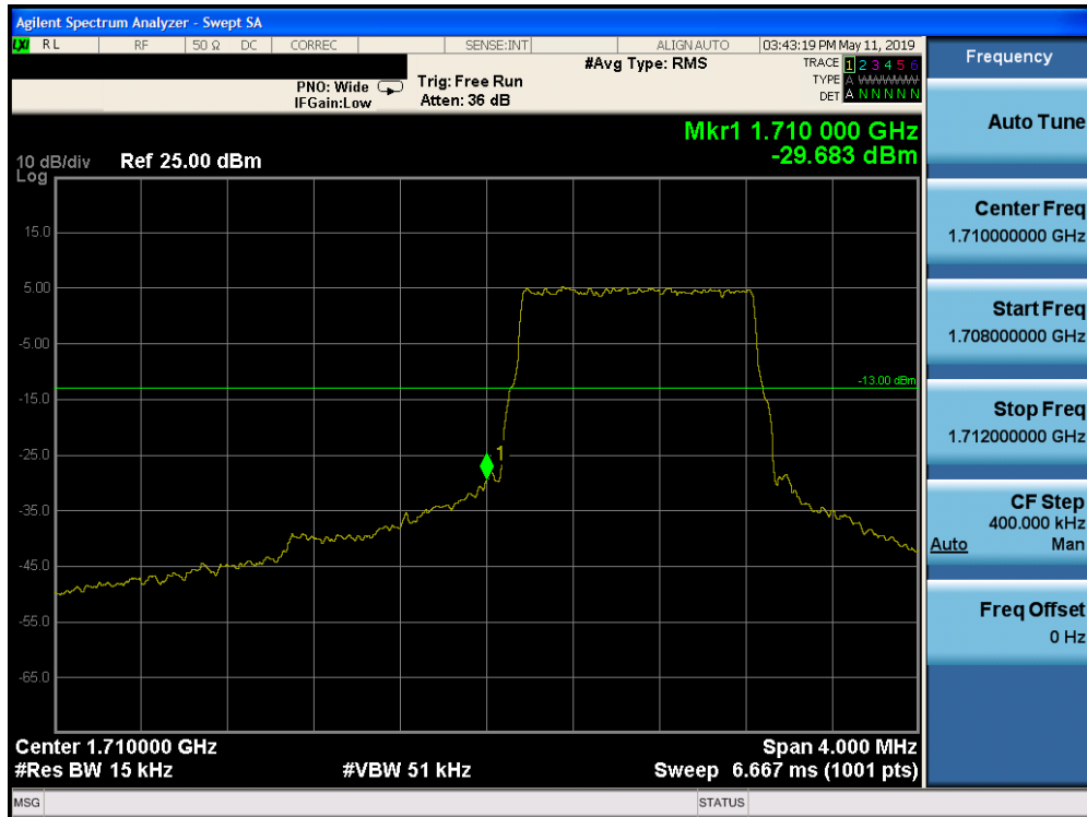
Plot 7-110. Lower Band Edge Plot (Band 66 - 1.4MHz QPSK - Full RB Configuration)
