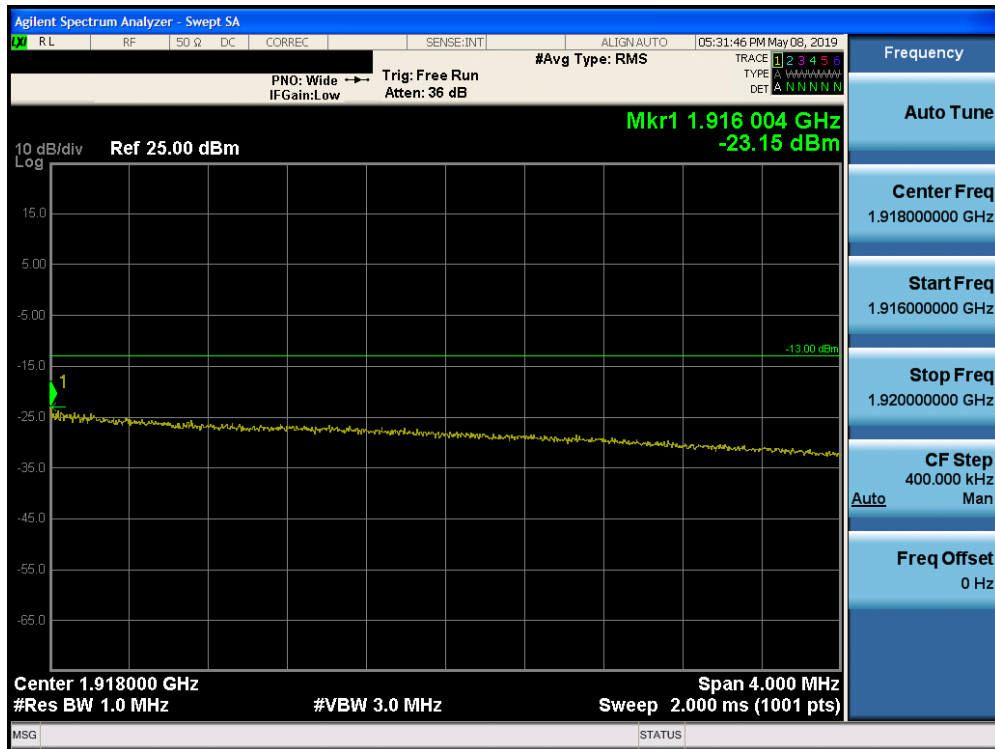
Plot 7-181. Upper Extended Band Edge Plot (Band 25 - 20.0MHz QPSK - Full RB Configuration)
