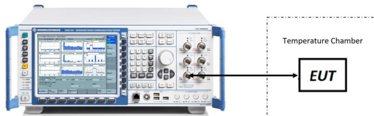
Figure 7-7. Test Instrument & Measurement Setup
