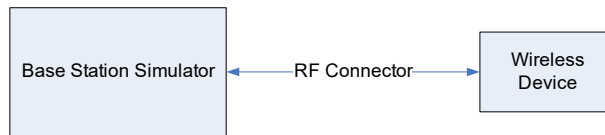
Figure 8-1 Power Measurement Setup
