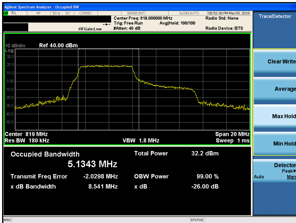
Plot 7-8. Occupied Bandwidth Plot (LTE Band 26, 10MHz 16-QAM – RB Size 27, RB Offset 0)
