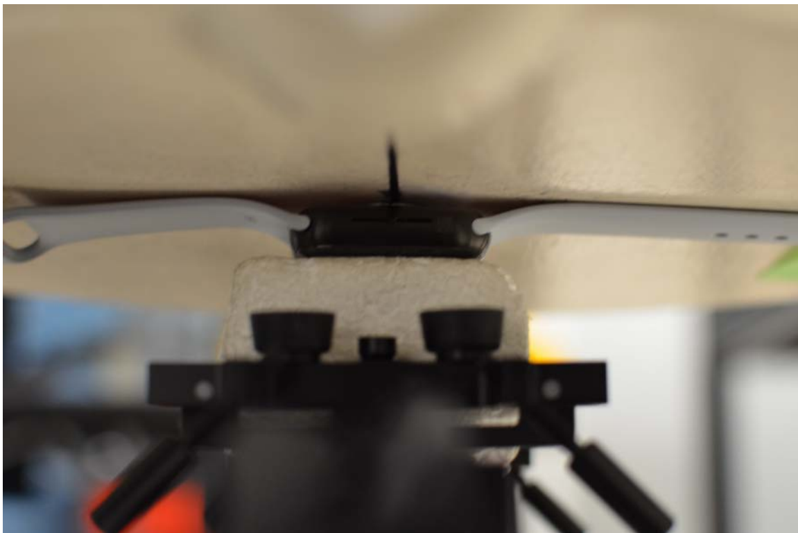
SAR Test Setup Photo 4: Aluminum with Sport Wristband, Back side at 0.0 cm
