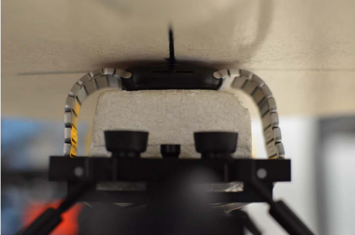
SAR Test Setup Photo 5: Aluminum with Metal Links Wristband, Back side at 0.0 cm
