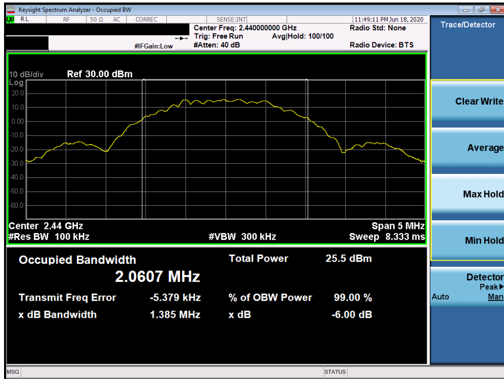
Plot 7-5. 6dB Bandwidth Plot (Bluetooth (LE), 2Mbps, ePA – Ch. 19)
