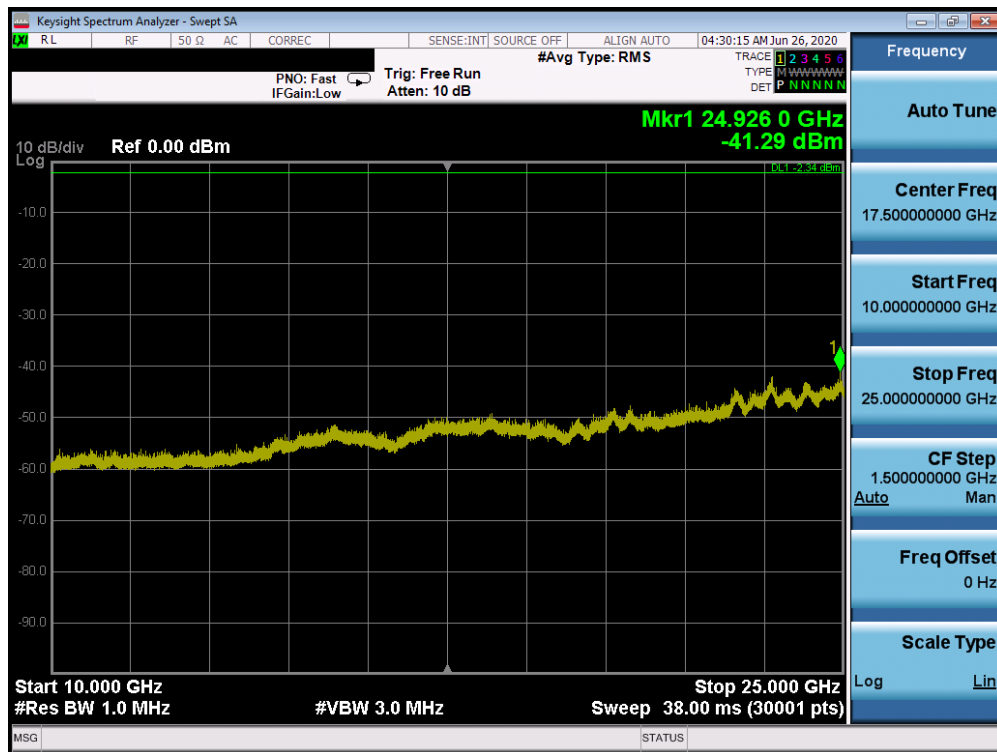
Plot 7-26. Conducted Spurious Plot (Bluetooth (LE), 1Mbps, ePA – Ch. 19)
