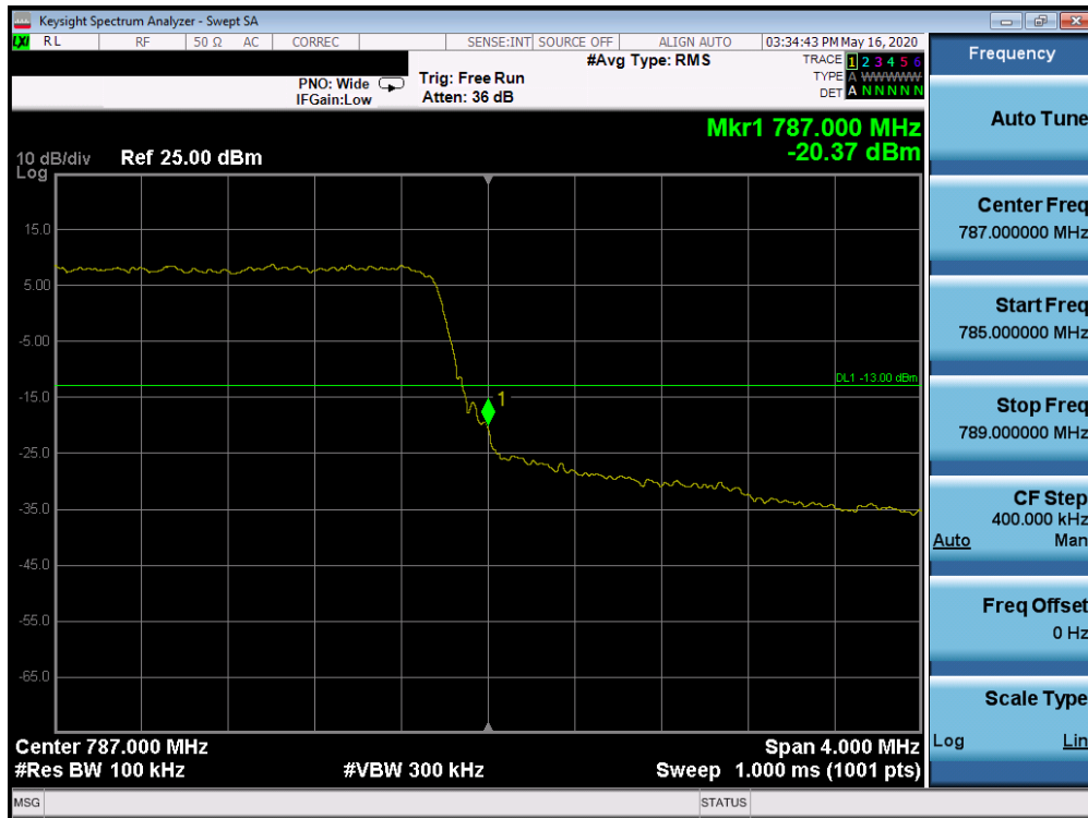
Plot 7-138. Upper Band Edge Plot (Band 13 - 5.0MHz QPSK - Full RB Configuration)
