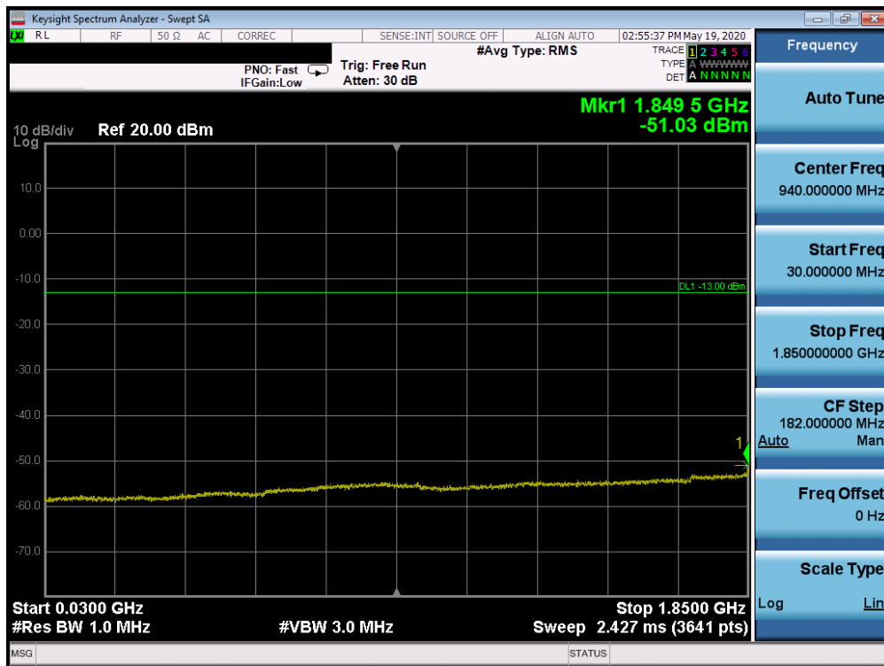
Plot 7-100. Conducted Spurious Plot (Band 25/2 - 20.0MHz QPSK - RB Size 1, RB Offset 0 - Mid Channel)
