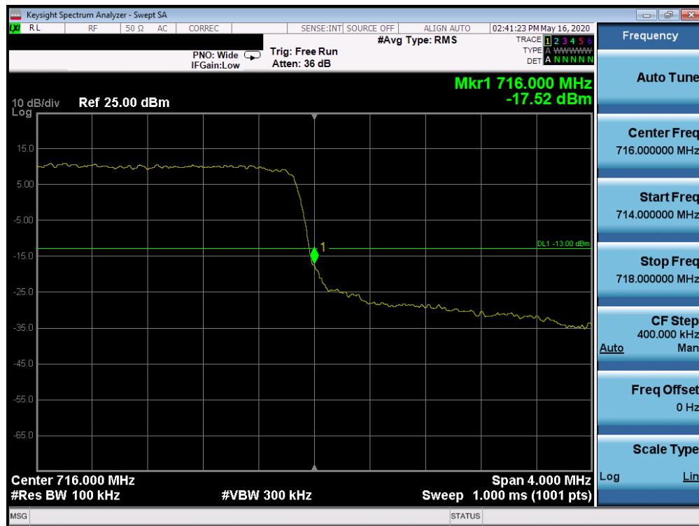
Plot 7-127. Upper Band Edge Plot (Band 12 - 3.0MHz QPSK - Full RB Configuration)
