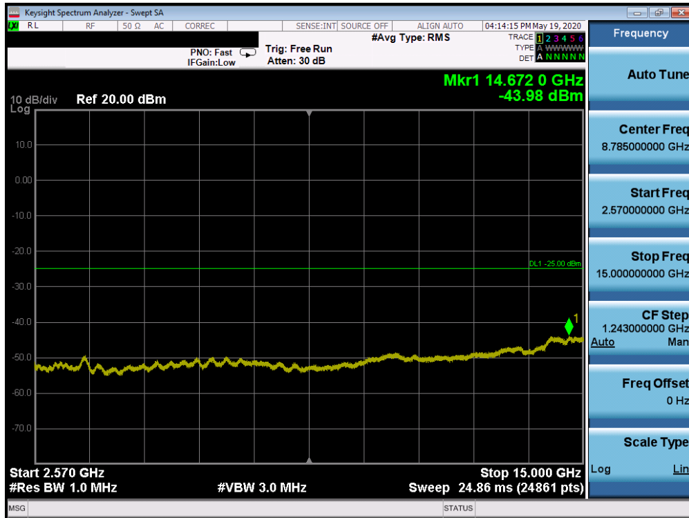
Plot 7-110. Conducted Spurious Plot (Band 7 - 20.0MHz QPSK - RB Size 1, RB Offset 0 - Mid Channel)
