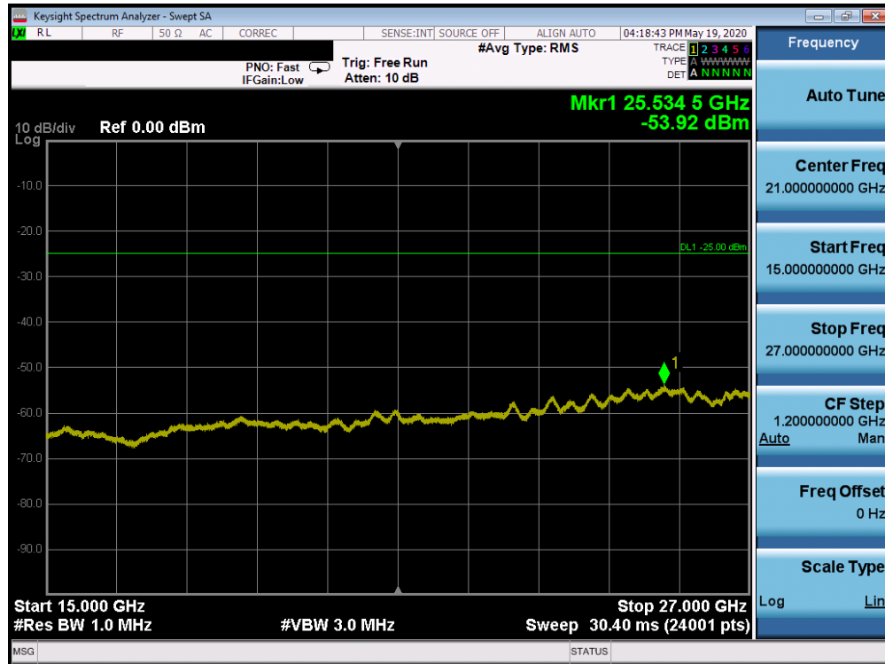
Plot 7-114. Conducted Spurious Plot (Band 7 - 20.0MHz QPSK - RB Size 1, RB Offset 0 - High Channel)
