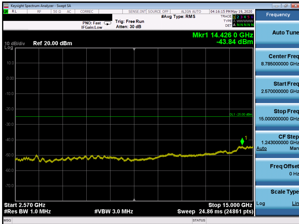
Plot 7-107. Conducted Spurious Plot (Band 7 - 20.0MHz QPSK - RB Size 1, RB Offset 0 - Low Channel)
