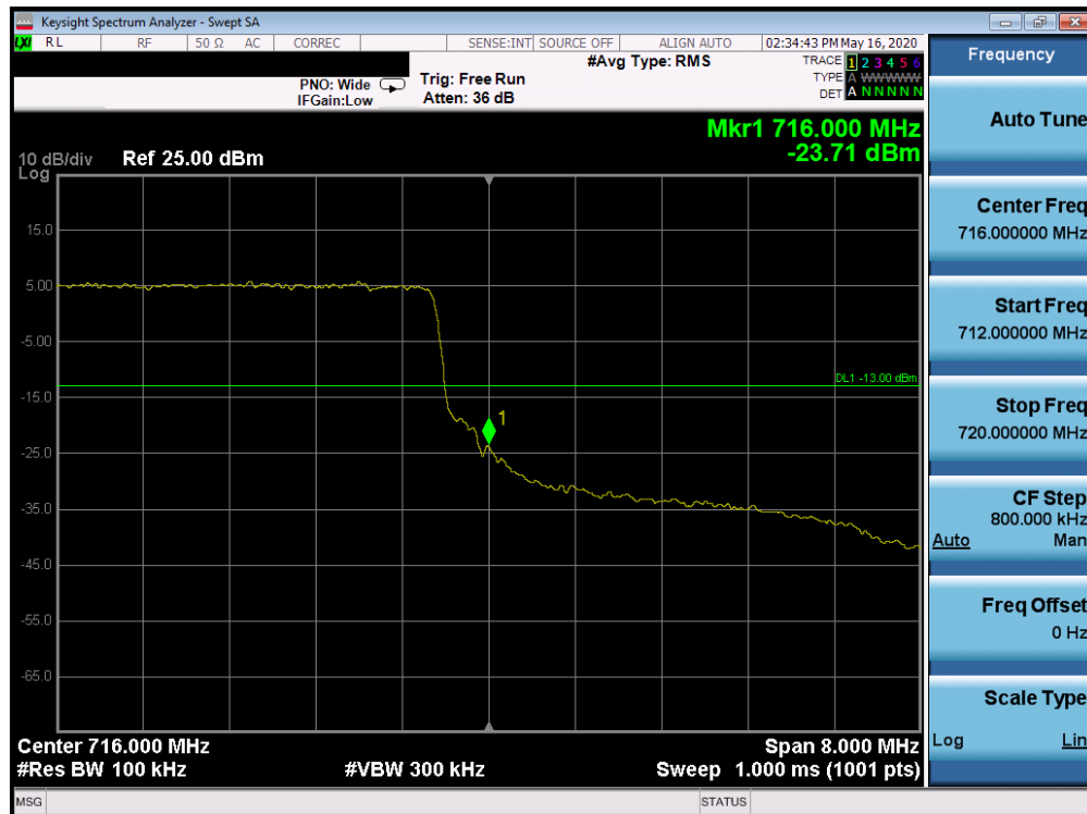
Plot 7-131. Upper Band Edge Plot (Band 12 - 10.0MHz QPSK - Full RB Configuration)
