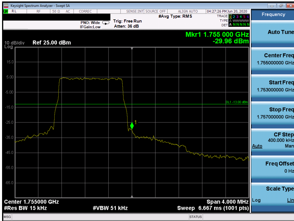
Plot 7-186. Upper Band Edge Plot (Band 4 - 1.4MHz QPSK - Full RB Configuration)
