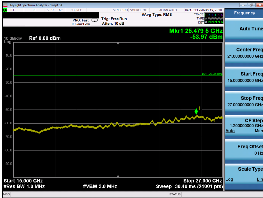
Plot 7-108. Conducted Spurious Plot (Band 7 - 20.0MHz QPSK - RB Size 1, RB Offset 0 - Low Channel)
