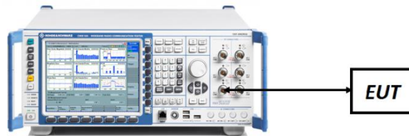
Figure 7-5. ERP/EIRP Measurement Setup
