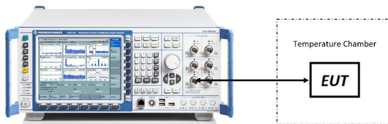
Figure 7-8. Test Instrument & Measurement Setup
