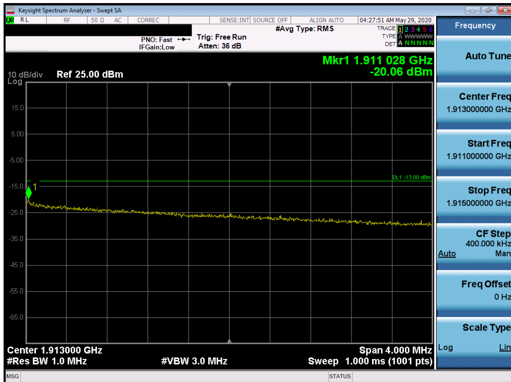
Plot 7-197. Upper Extended Band Edge Plot (Band 2 - 10.0MHz QPSK - Full RB Configuration)
