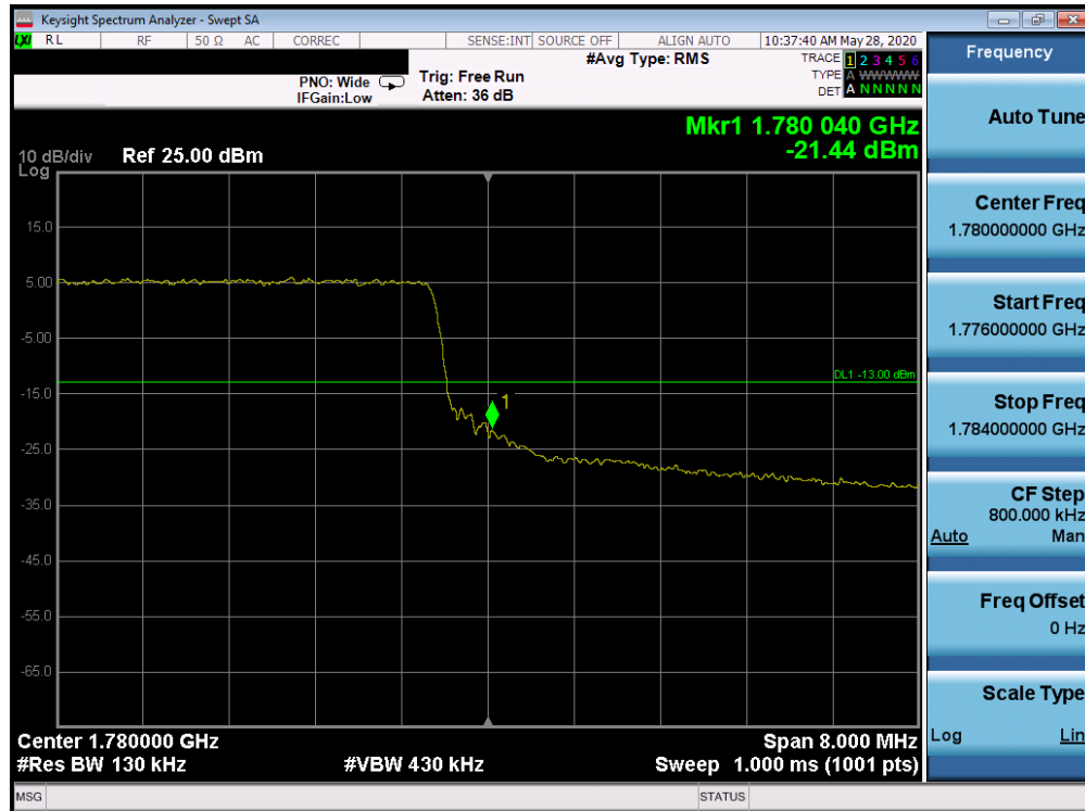
Plot 7-124. Upper Band Edge Plot (Band 66 - 10.0MHz QPSK - Full RB Configuration)
