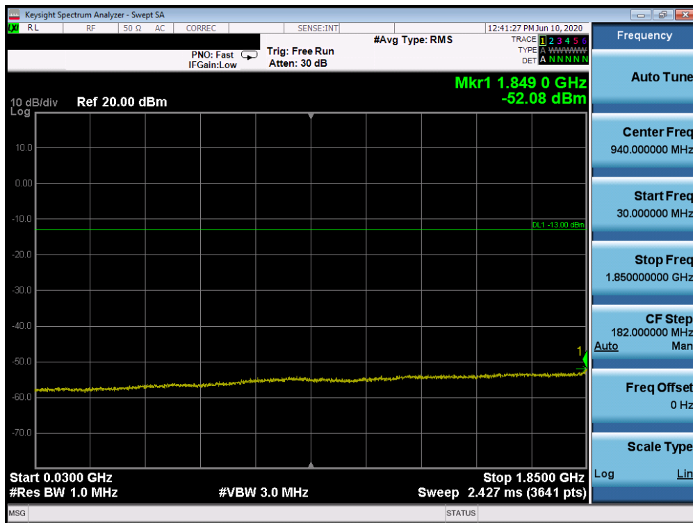
Plot 7-25. Conducted Spurious Plot (PCS WCDMA Mode - Mid Channel)
