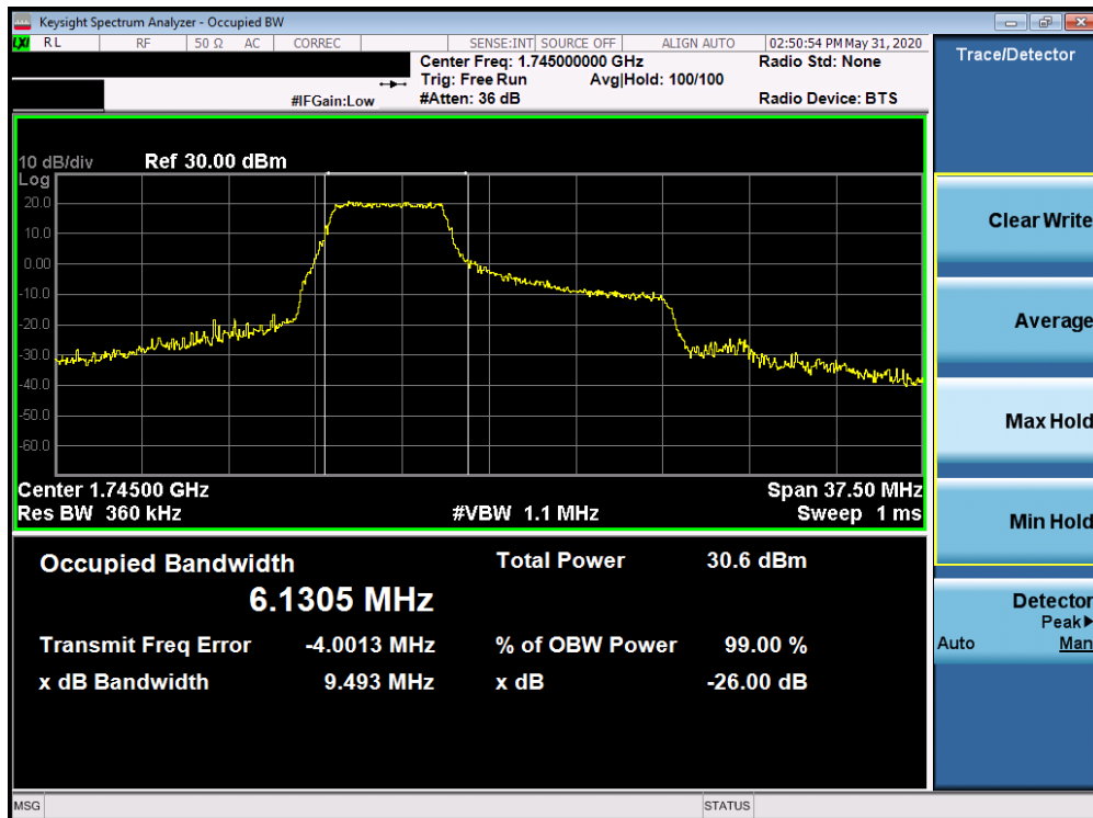
Plot 7-18. Occupied Bandwidth Plot (Band 66/4 - 15.0MHz 16-QAM - Full RB Configuration)
