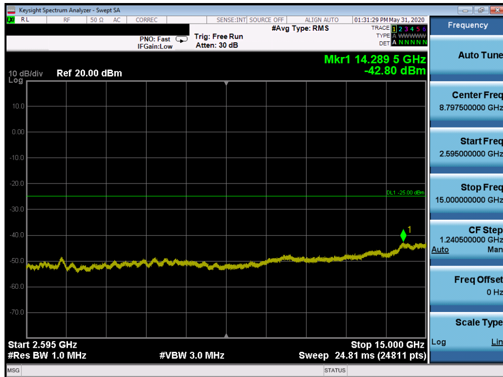
Plot 7-83. Conducted Spurious Plot (Band 7 - 20.0MHz QPSK - RB Size 1, RB Offset 0 - High Channel)
