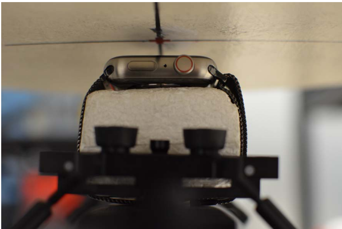
SAR Test Setup Photo 9: Titanium with Metal Loop Wristband, Front Side at 1.0 cm
