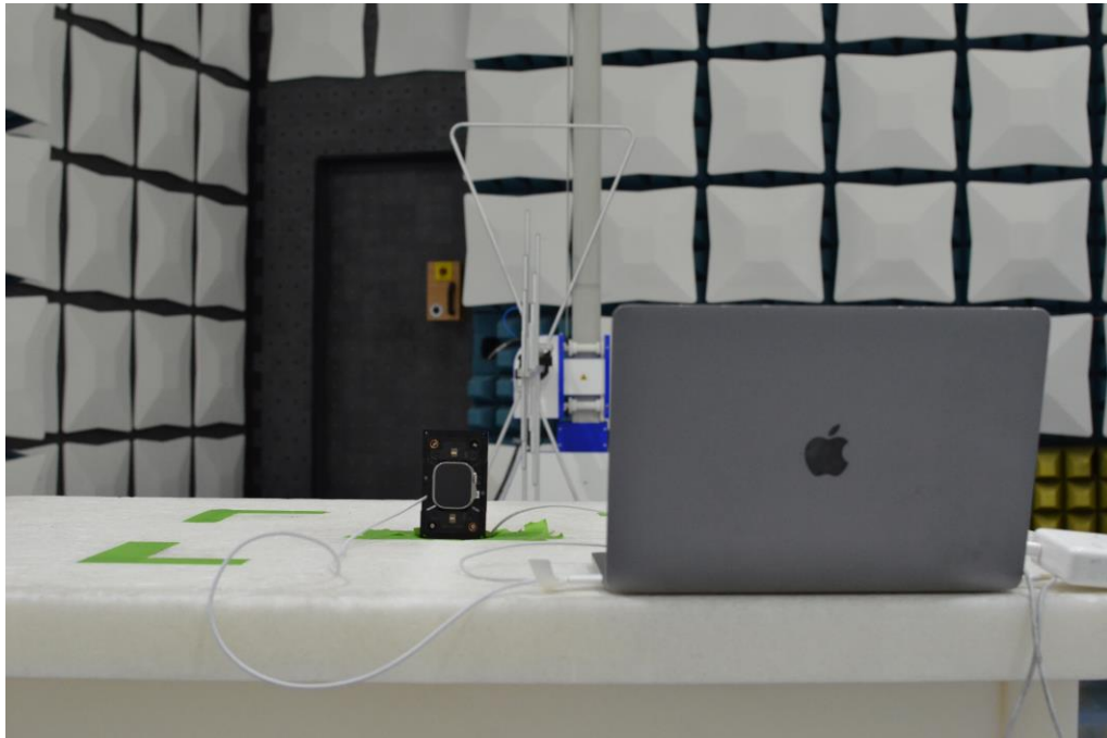
Figure 17: 30MHz-1GHz Test Setup (Rear View)
