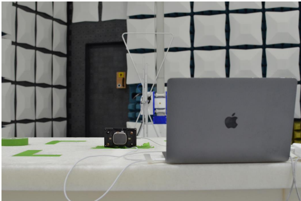
Figure 15: 30MHz-1GHz Test Setup (Rear View)
