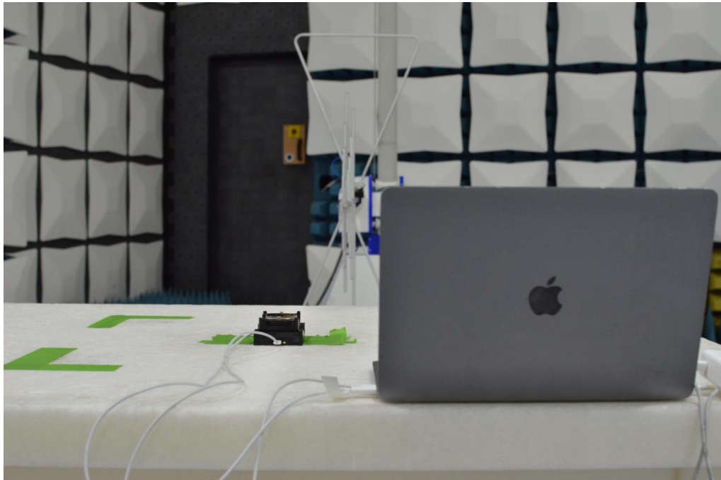
Figure 13: 30MHz-1GHz Test Setup (Rear View)
