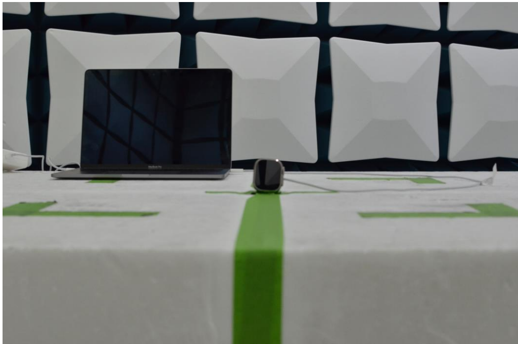
Figure 17: 30MHz-1GHz Test Setup (Front View)
