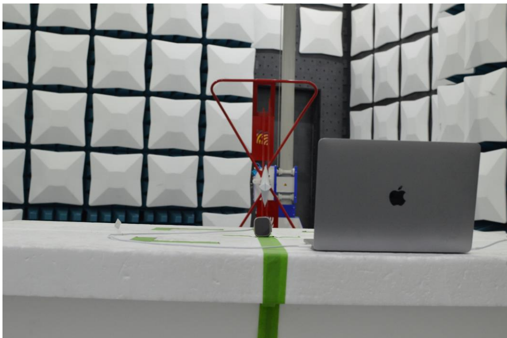
Figure 18: 30MHz-1GHz Test Setup (Rear View)
