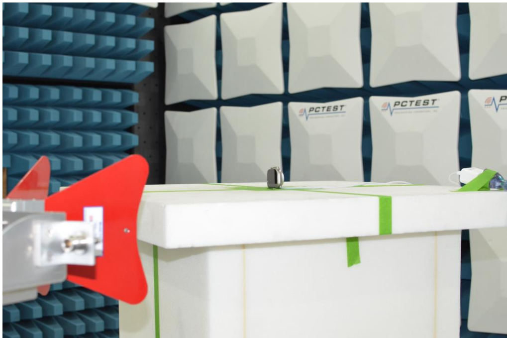
Figure 6: Above 960MHz Test Setup
