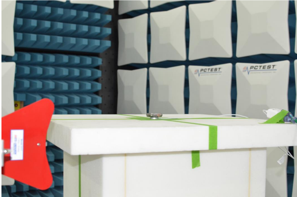
Figure 5: Above 960MHz Test Setup
