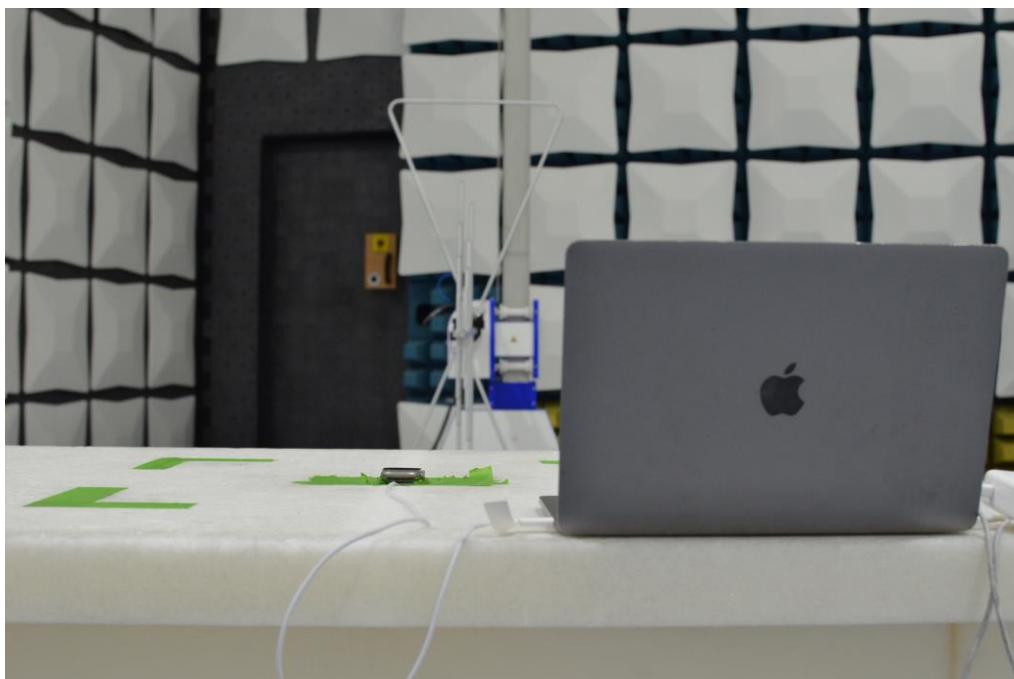
Figure 18: 30MHz-1GHz Test Setup (Rear View)
