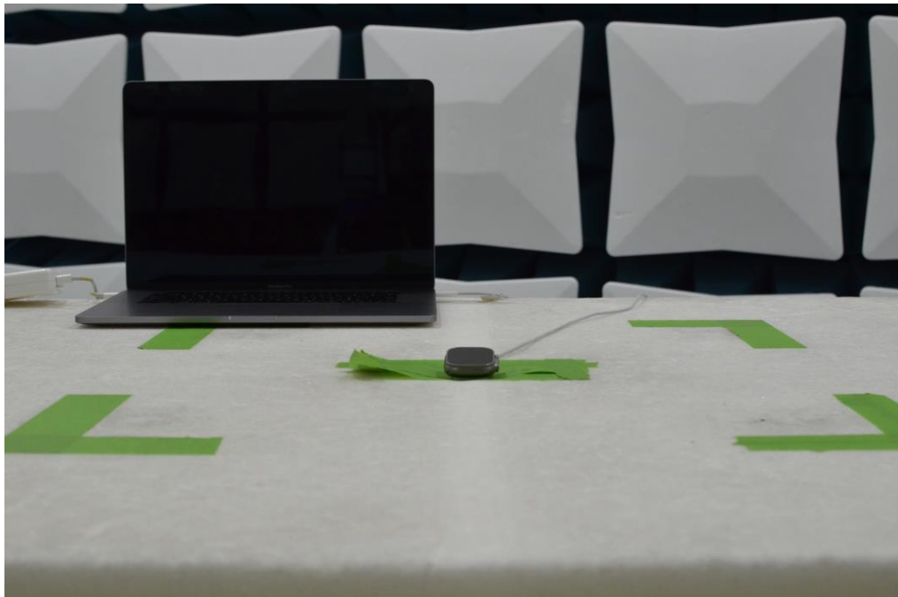
Figure 17: 30MHz-1GHz Test Setup (Front View)
