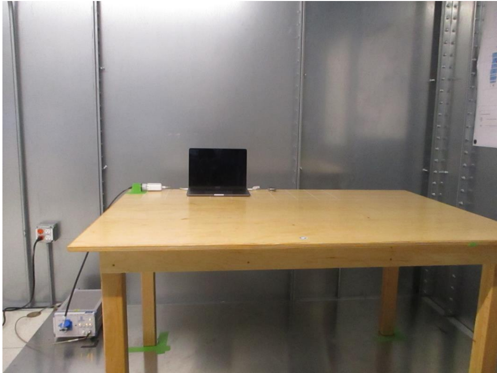
Figure 3: AC Line Conducted Emissions (Front View)
