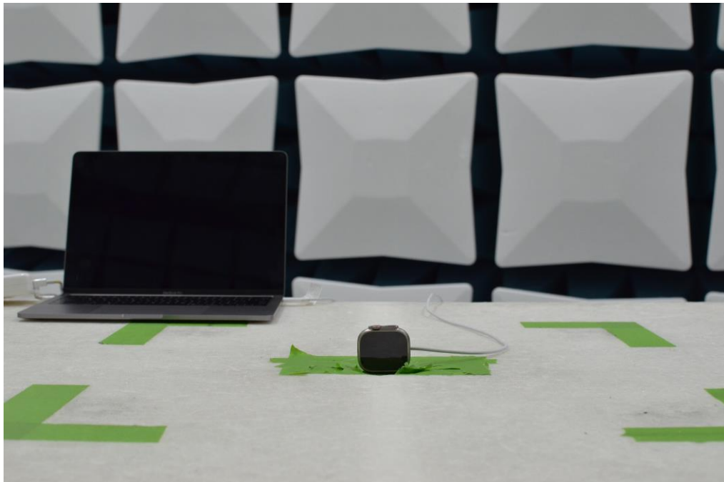
Figure 19: 30MHz-1GHz Test Setup (Front View)
