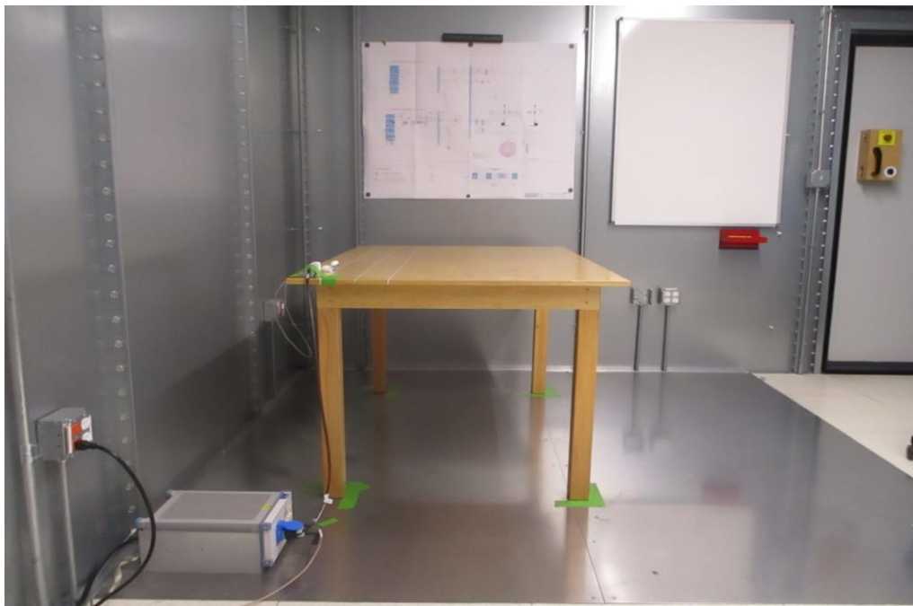
Figure 2: AC Line Conducted Emissions (Side View)
