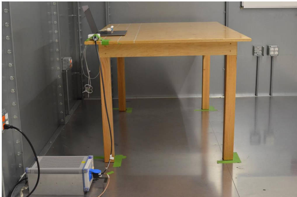
Figure 4: AC Line Conducted Emissions (Side View)
