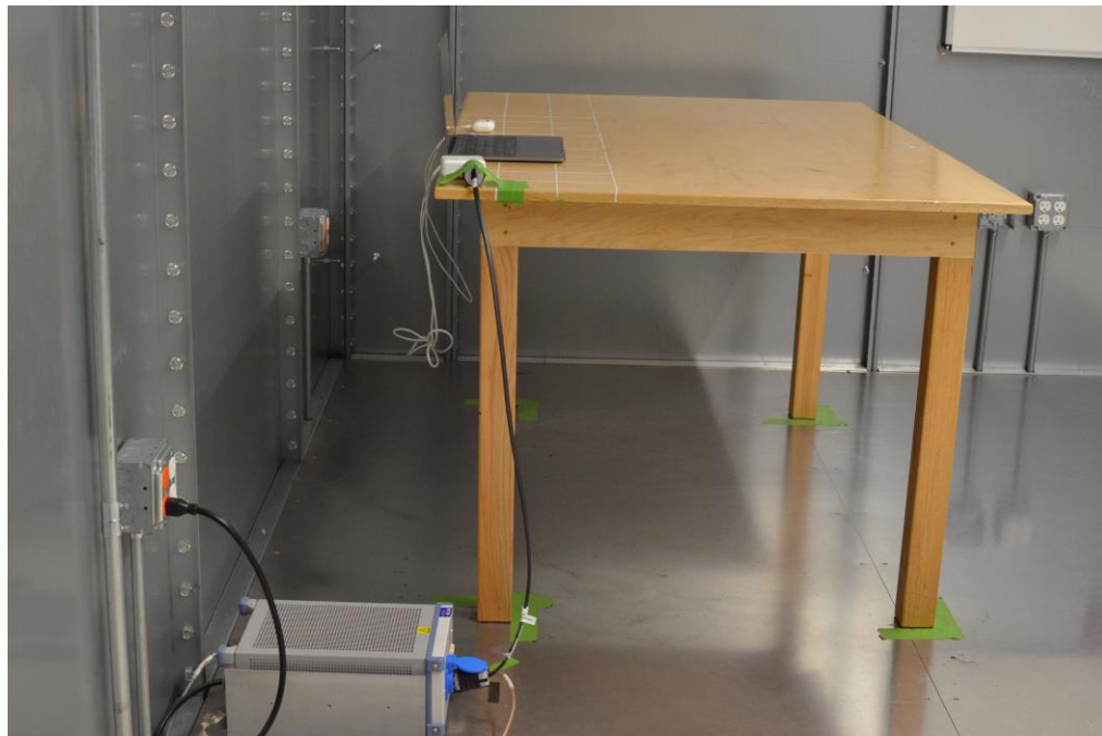
Figure 4: AC Line Conducted Emissions (Side View)
