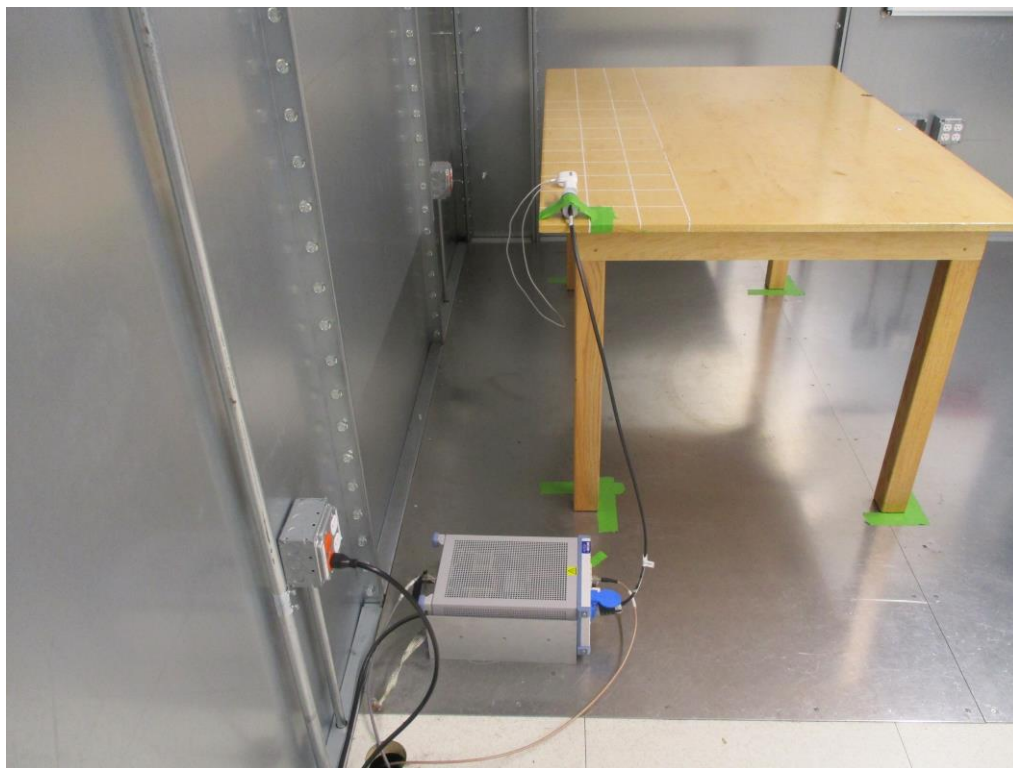
Figure 2: AC Line Conducted Emissions (Side View)
