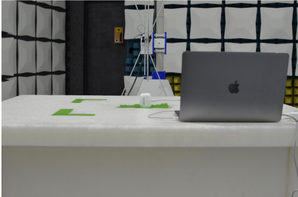
Figure 17: 30MHz-1GHz Test Setup (Rear View)
