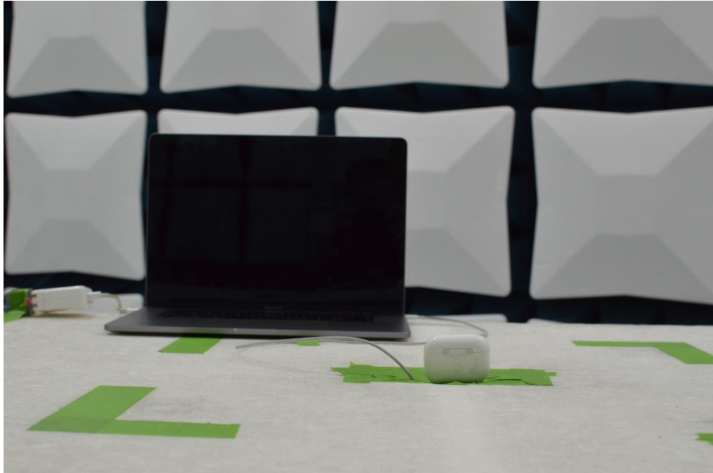
Figure 21: 30MHz-1GHz Test Setup (Front View)
