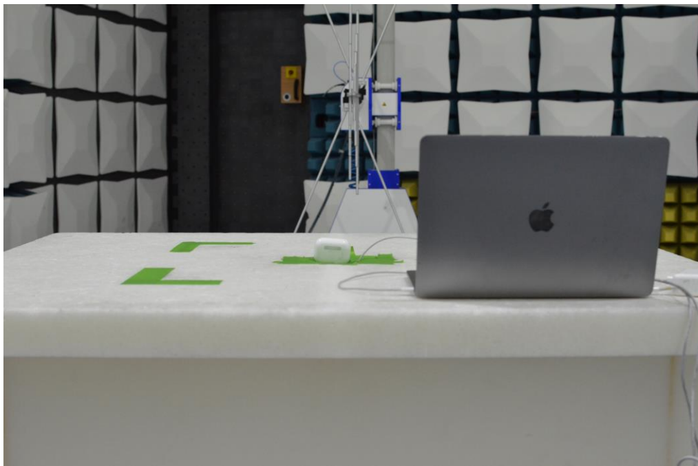
Figure 22: 30MHz-1GHz Test Setup (Rear View)
