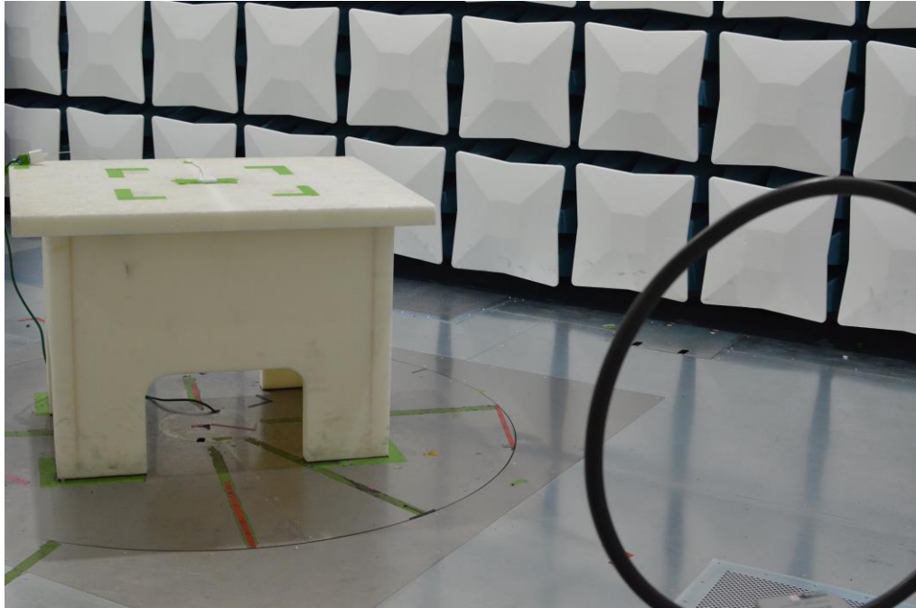
Figure 23: 9kHz-30MHz Test Setup (Front View)
