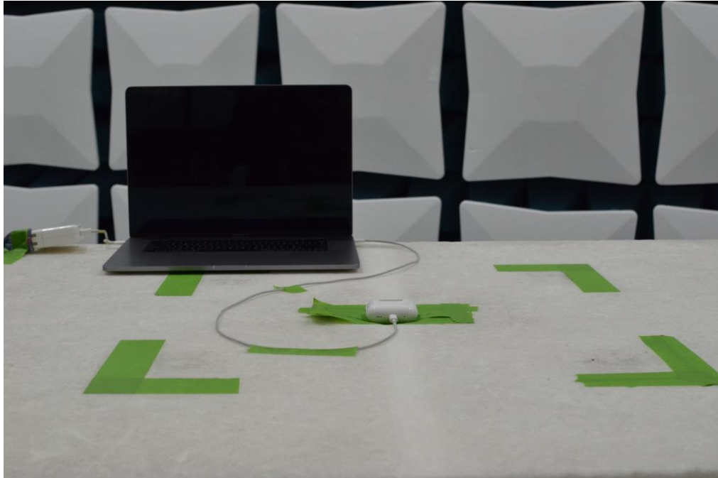
Figure 17: 30MHz-1GHz Test Setup (Front View)
