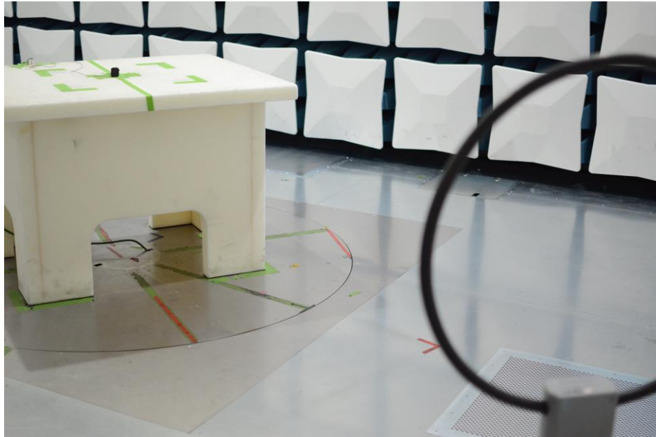
Figure 25: 9kHz-30MHz Test Setup (Front View)
