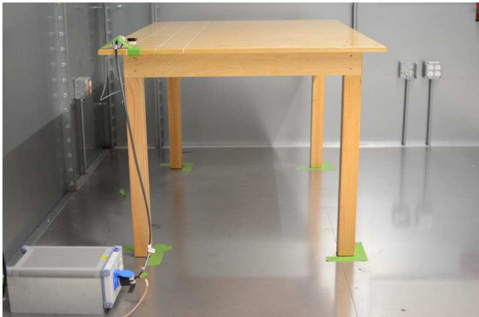
Figure 2: AC Line Conducted Emissions (Side View)
