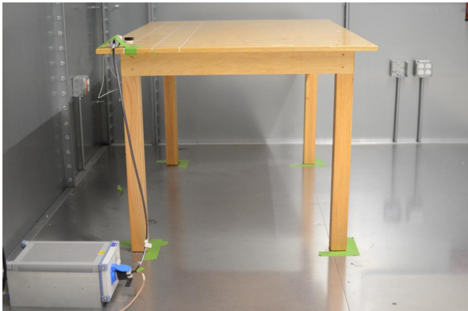
Figure 2: AC Line Conducted Emissions (Side View)
