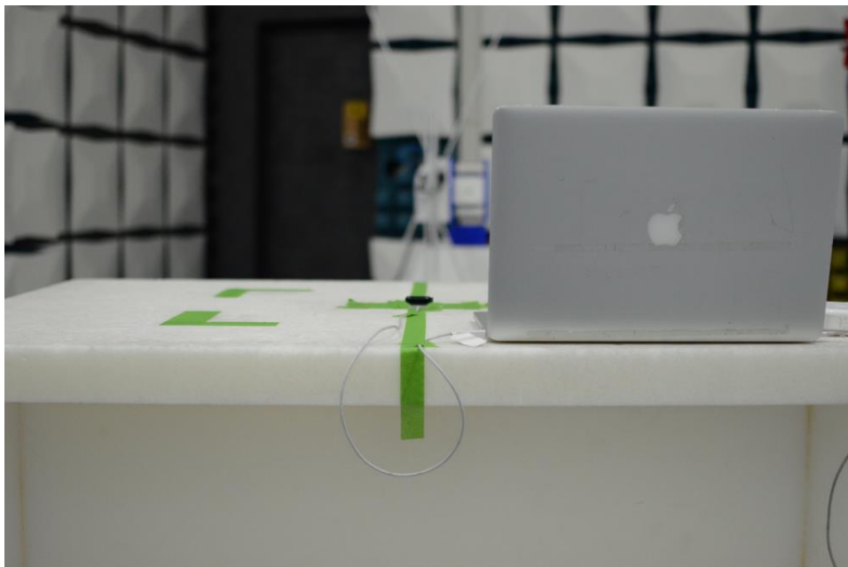
Figure 18: 30MHz-1GHz Test Setup (Rear View)
