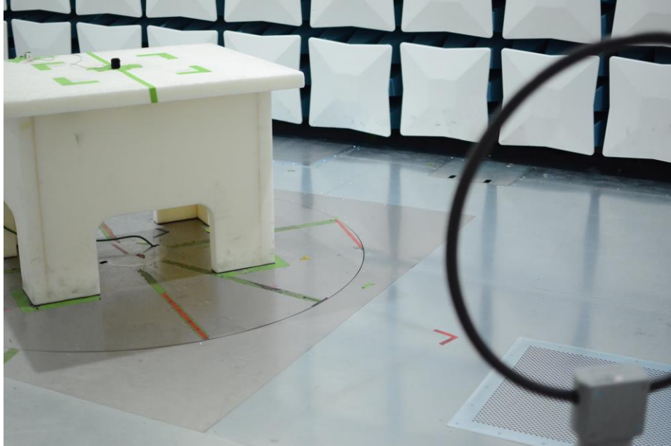
Figure 25: 9kHz-30MHz Test Setup (Front View)
