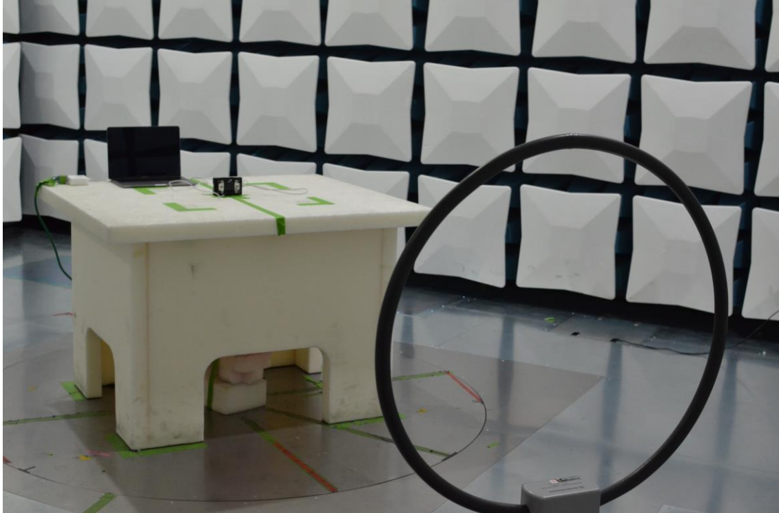
Figure 19: 9kHz-30MHz Test Setup (Front View)
