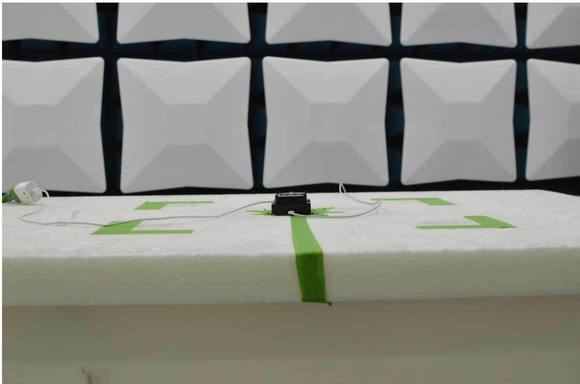
Figure 6: 1-18GHz Test Setup (Front View)
