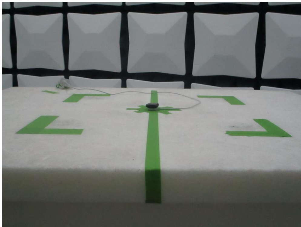
Figure 7: 30MHz-1GHz Test Setup (Front View)
