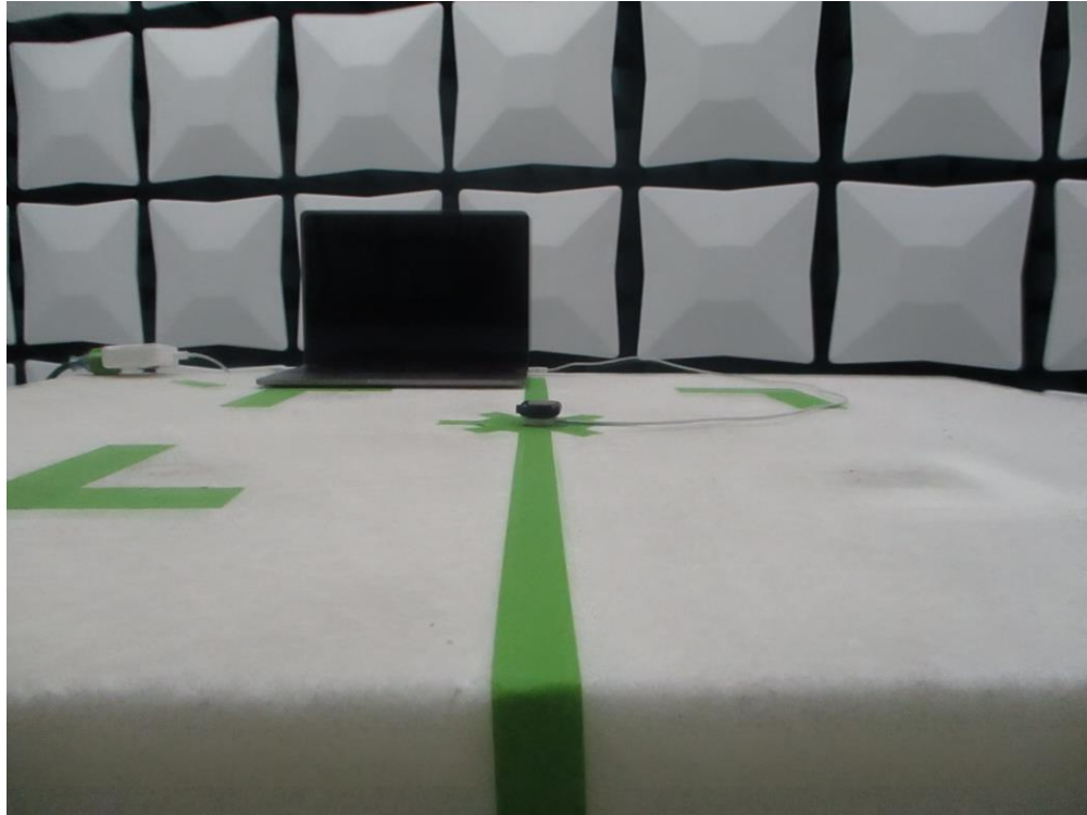
Figure 13: 30MHz-1GHz Test Setup (Front View)
