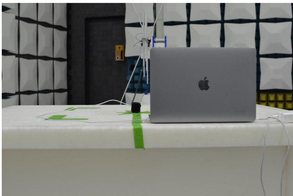
Figure 18: 30MHz-1GHz Test Setup (Rear View)
