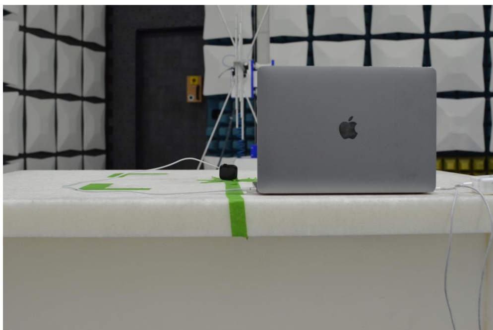
Figure 16: 30MHz-1GHz Test Setup (Rear View)
