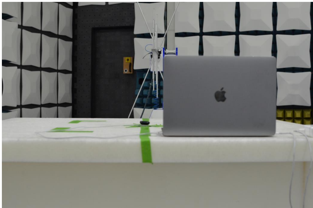
Figure 14: 30MHz-1GHz Test Setup (Rear View)
