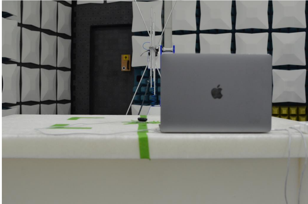
Figure 15: 30MHz-960MHz Test Setup (Rear View)
