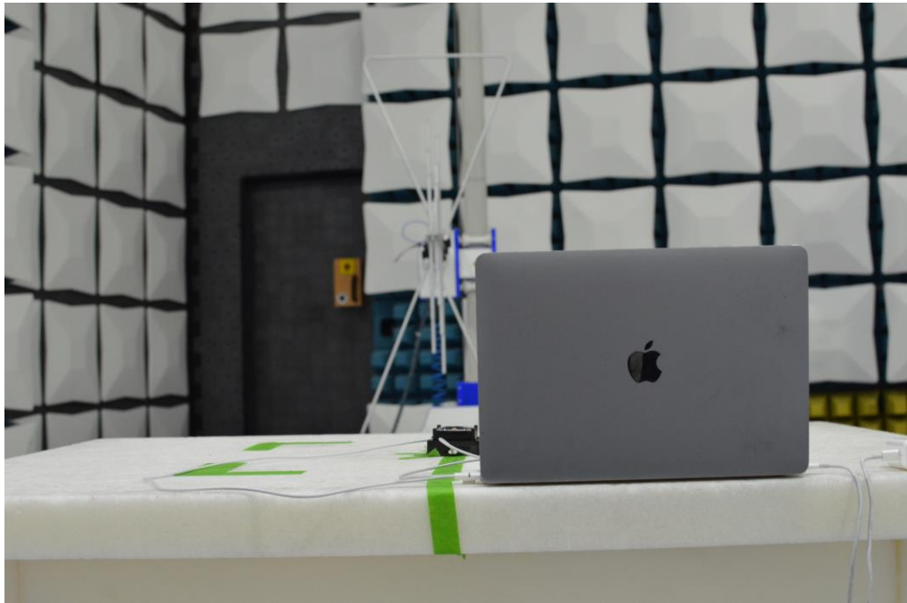
Figure 13: 30MHz-1GHz Test Setup (Rear View)
