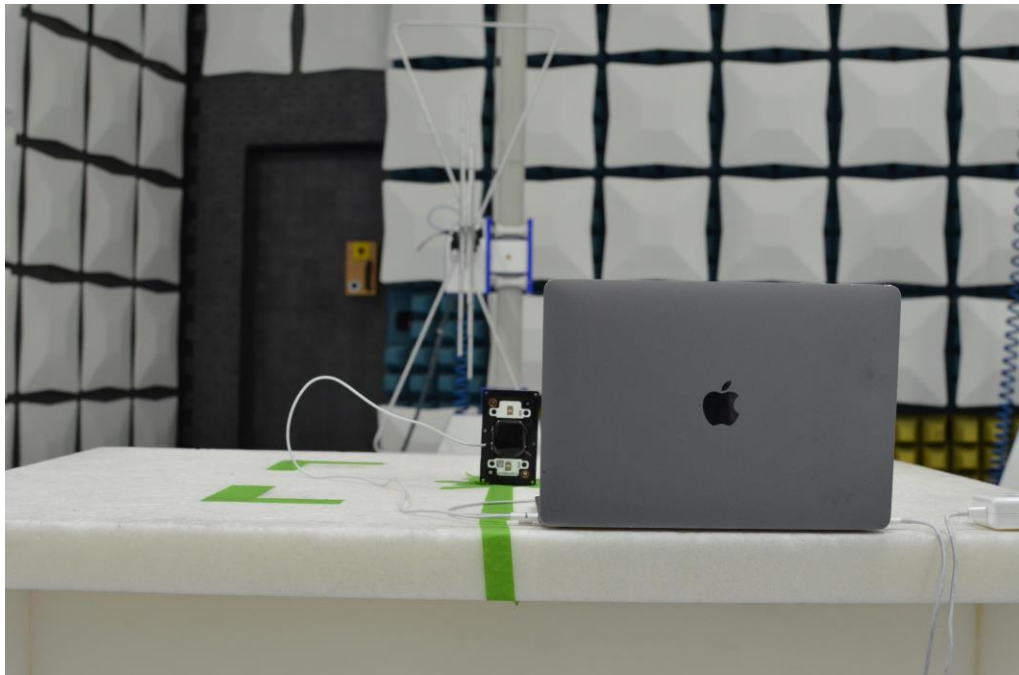
Figure 16: 30MHz-1GHz Test Setup (Front View)
