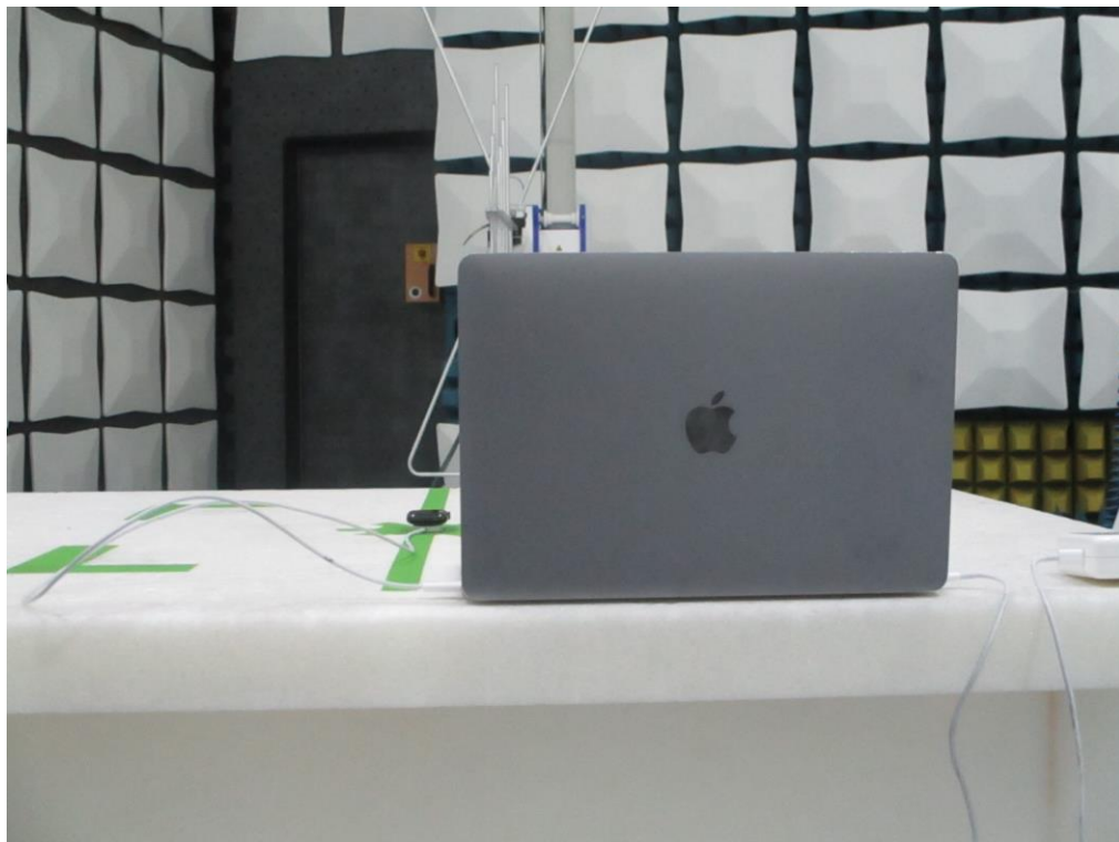
Figure 18: 30MHz-1GHz Test Setup (Rear View)
