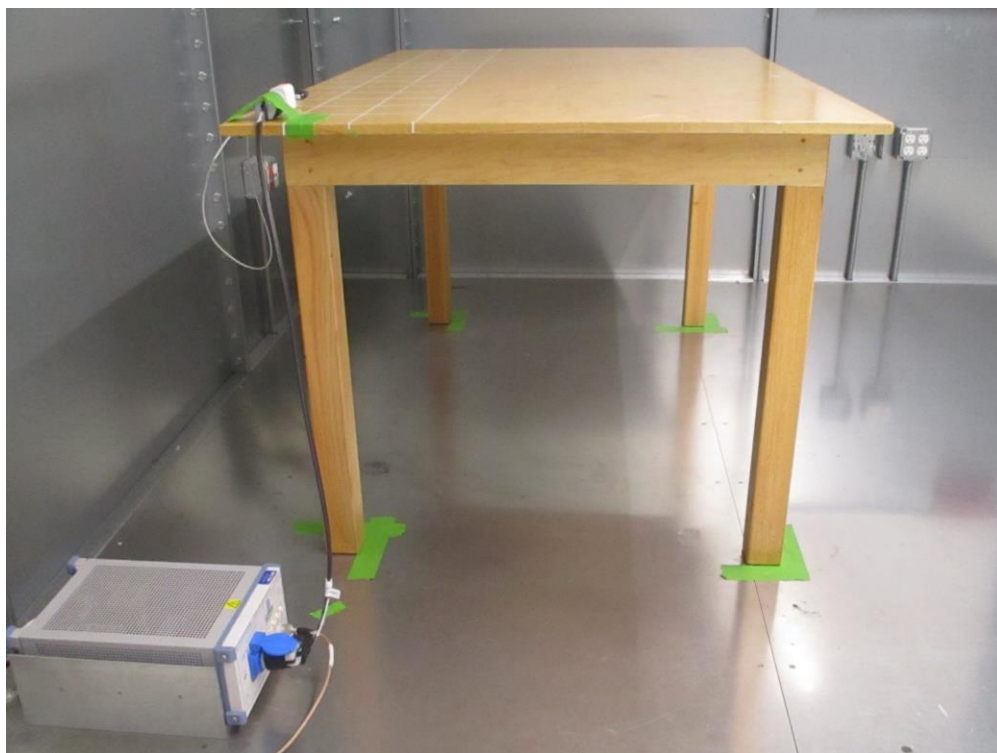
Figure 2: AC Line Conducted Emissions (Side View)
