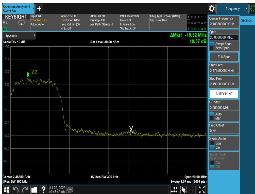
Plot 7-22. Band Edge Plot (Bluetooth (HDR8), ePA – Ch. 73)
