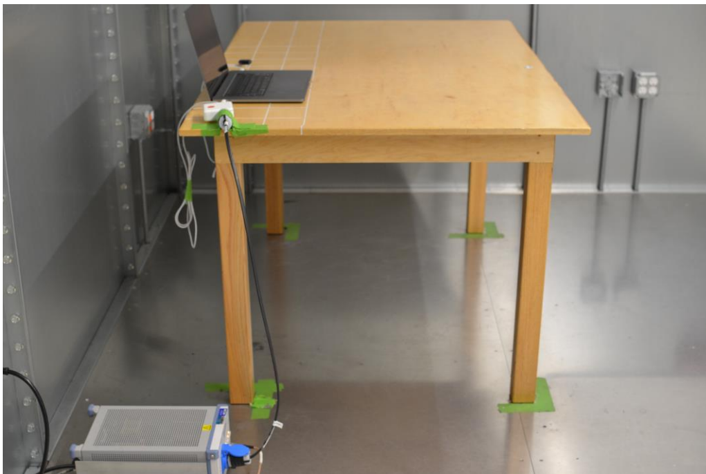
Figure 4: AC Line Conducted Emissions (Side View)
