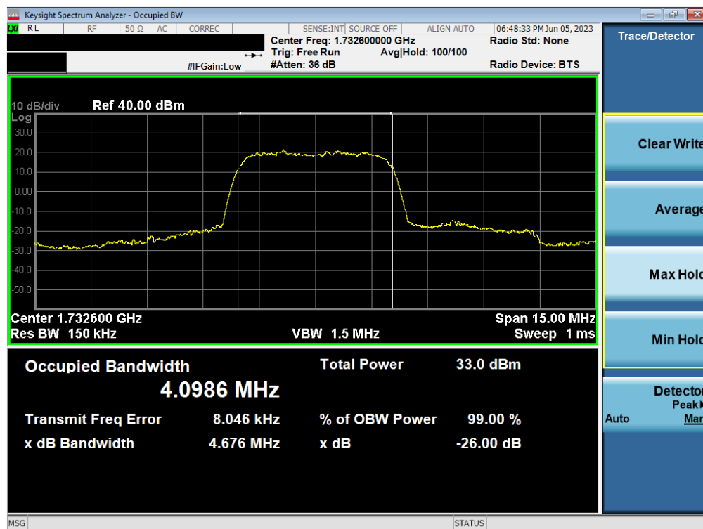
Plot 7-25. Occupied Bandwidth Plot (WCDMA, Ch. 1413)
