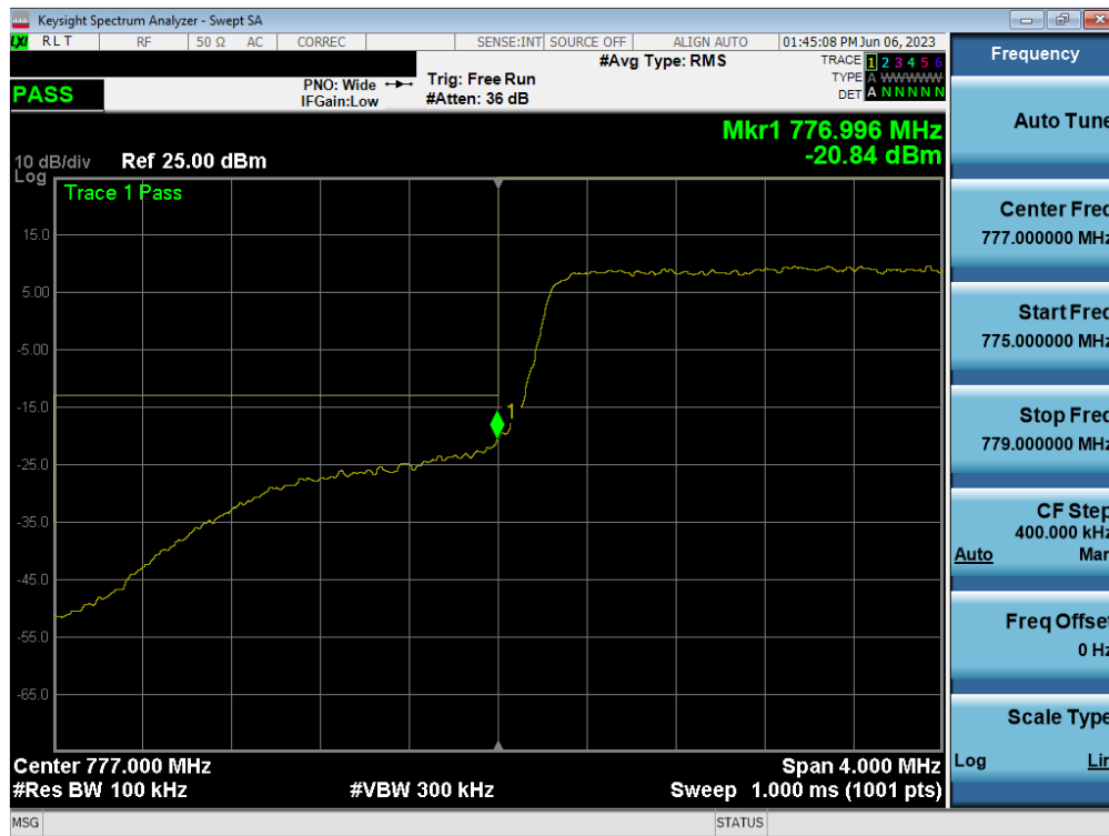
Plot 7-116. Lower Band Edge Plot (LTE Band 13 - 5MHz QPSK – Full RB)
