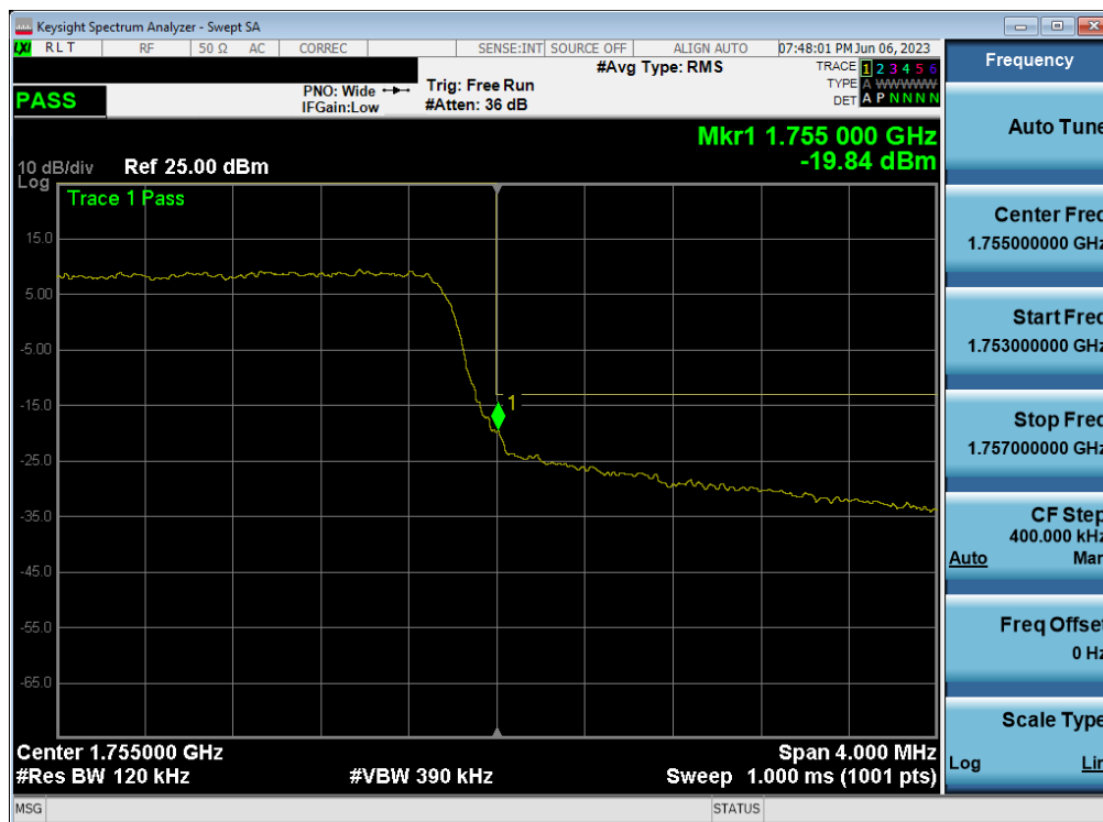
Plot 7-90. Upper Band Edge Plot (LTE Band 4 - 5MHz QPSK – Full RB)
