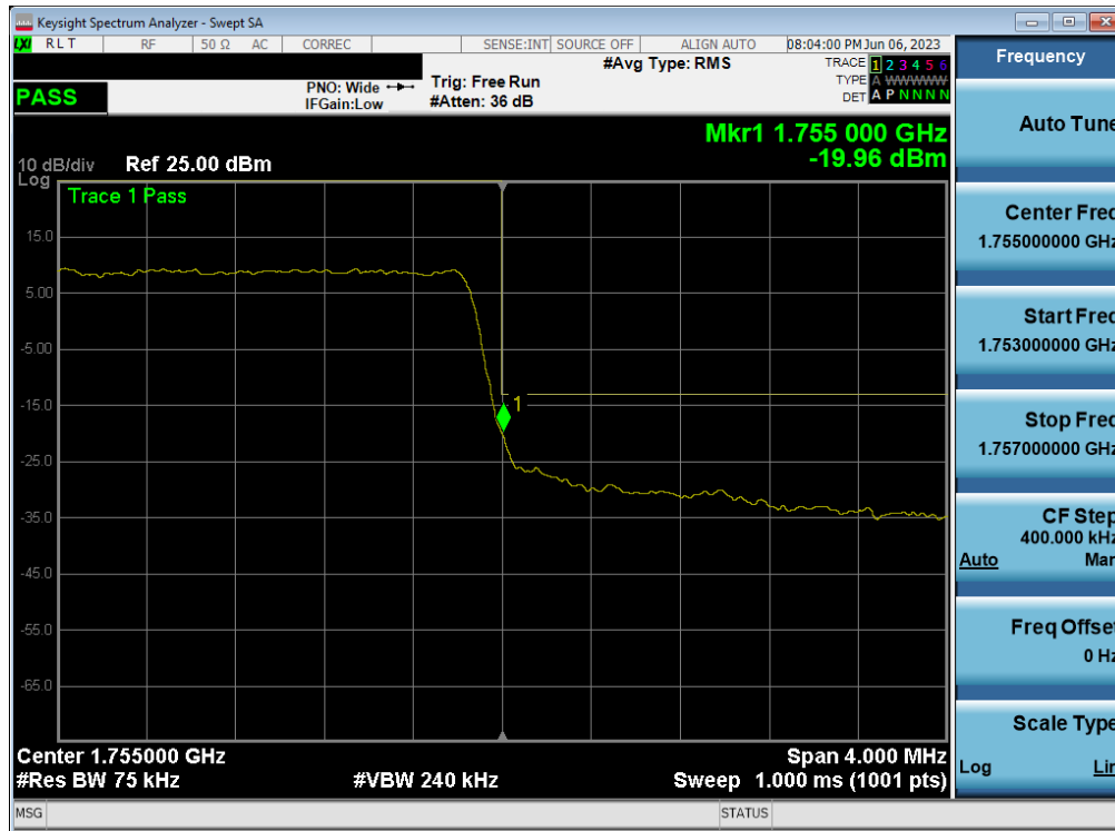
Plot 7-86. Upper Band Edge Plot (LTE Band 4 - 3MHz QPSK – Full RB)
