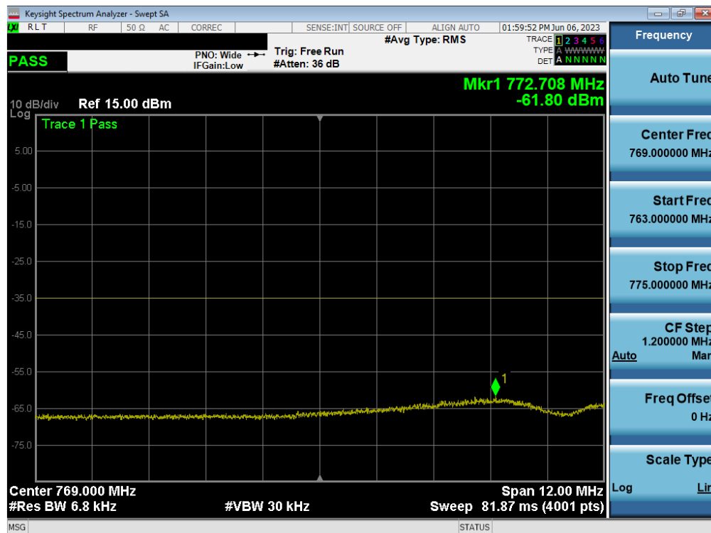
Plot 7-121. Lower Emission Mask Plot (LTE Band 13 - 10MHz QPSK – Full RB)
