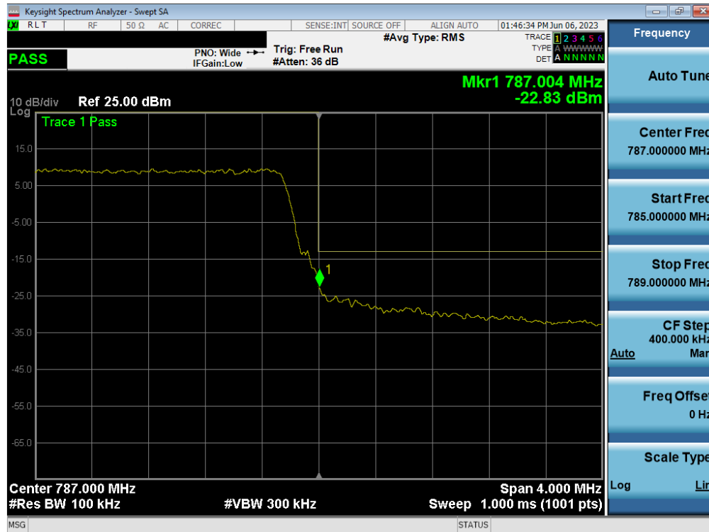
Plot 7-118. Upper Band Edge Plot (LTE Band 13 - 5MHz QPSK – Full RB)
