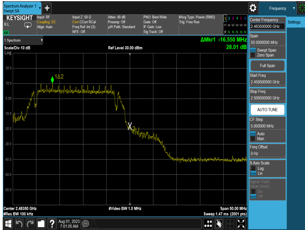
Plot 7-35. Band Edge Plot (802.11g – Ch. 13) – 6Mbps
