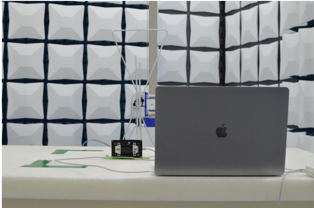
Figure 15: 30MHz-1GHz Test Setup (Rear View)
