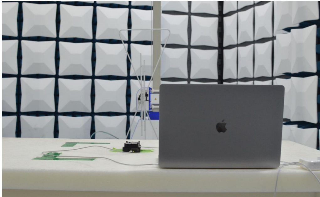
Figure 13: 30MHz-1GHz Test Setup (Rear View)
