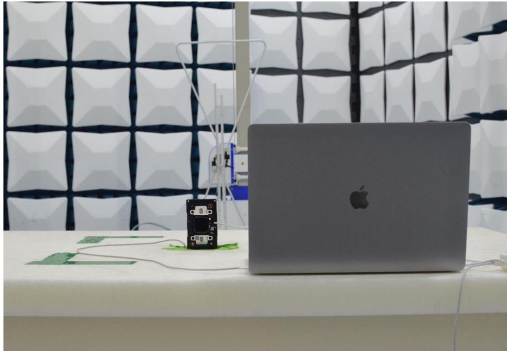
Figure 17: 30MHz-1GHz Test Setup (Rear View)
