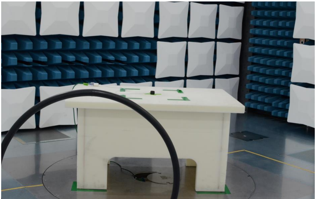
Figure 20: 9kHz-30MHz Test Setup (Front View)
