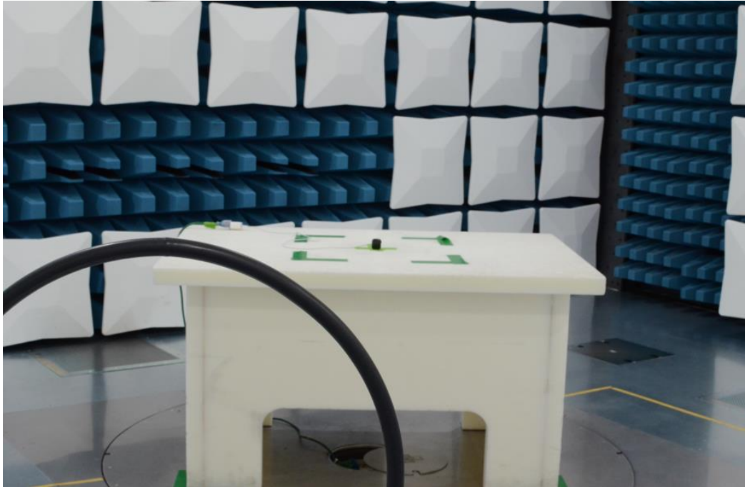
Figure 21: 9kHz-30MHz Test Setup (Front View)
