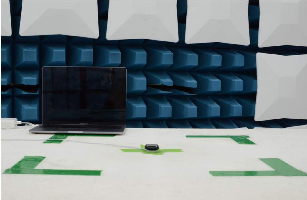
Figure 13: 30MHz-1GHz Test Setup (Front View)
