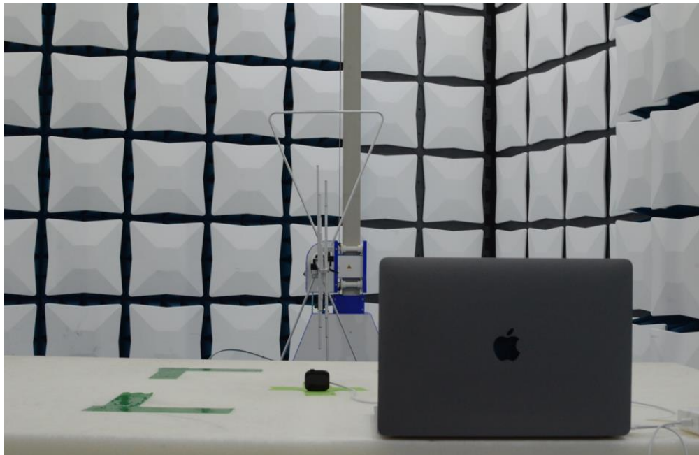
Figure 16: 30MHz-1GHz Test Setup (Rear View)
