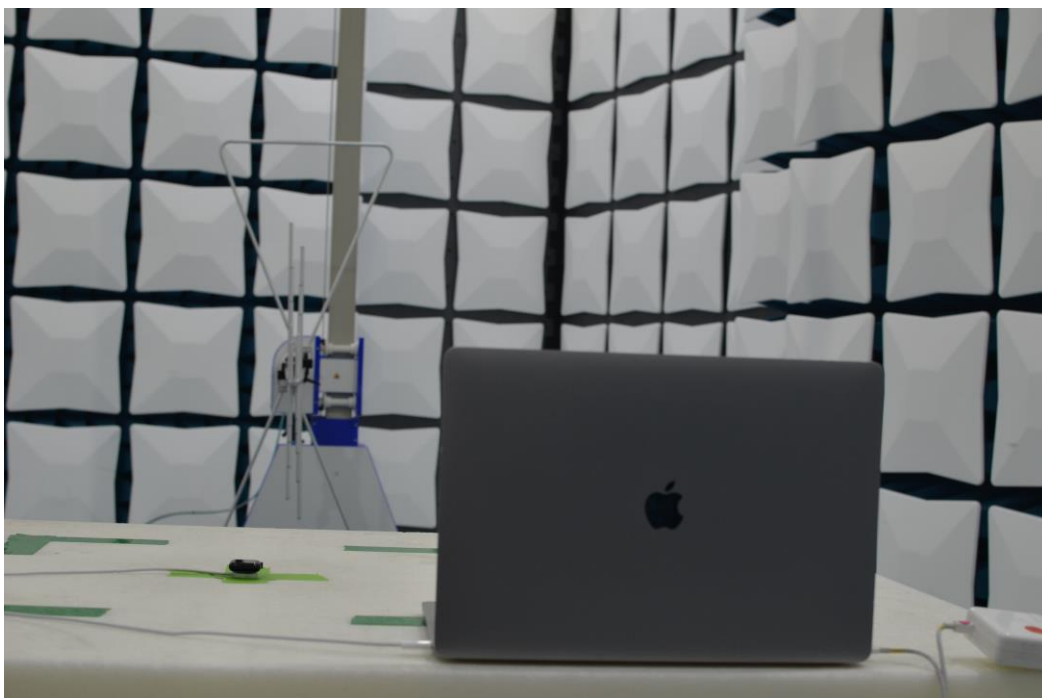
Figure 14: 30MHz-1GHz Test Setup (Rear View)
