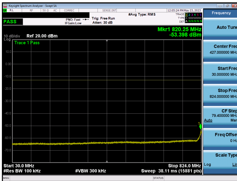
Plot 7-13. Conducted Spurious Plot (LTE Band 26/5 - 10MHz QPSK - RB Size 1, RB Offset 0 - Mid Channel)
