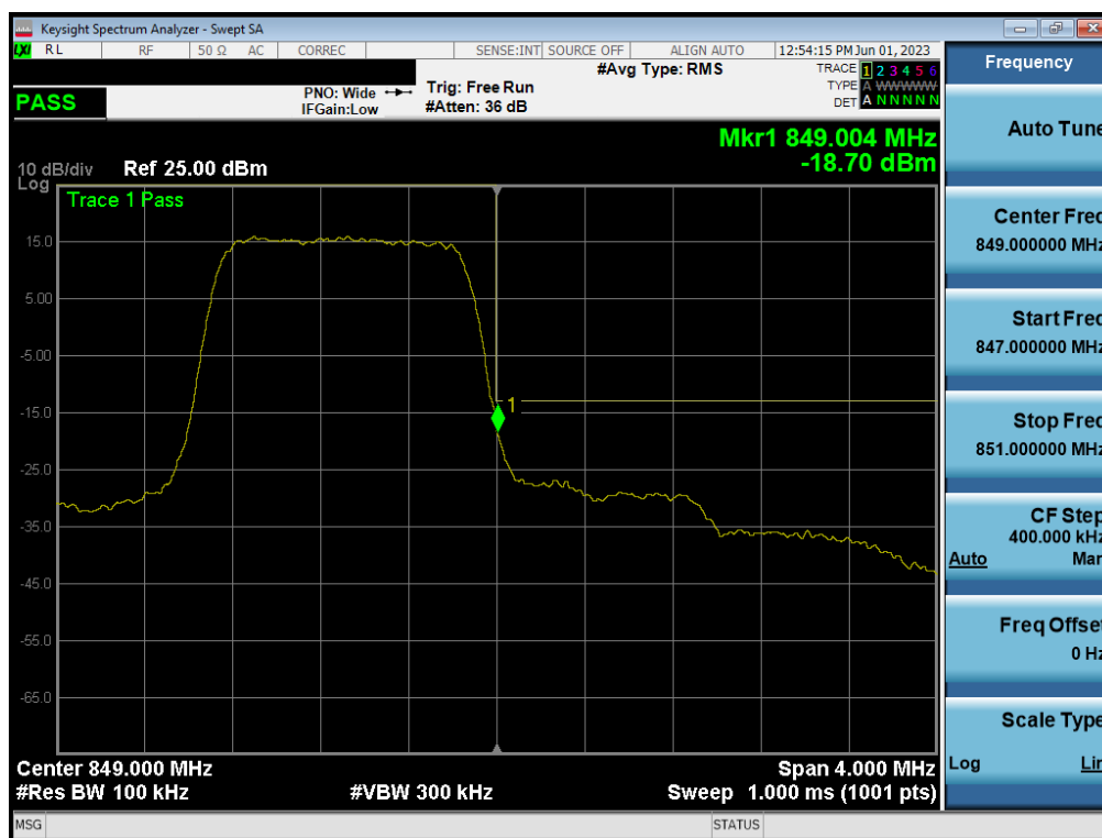
Plot 7-29. Upper BE Plot (LTE Band 26 – 1.4MHz QPSK – Full RB Configuration)
