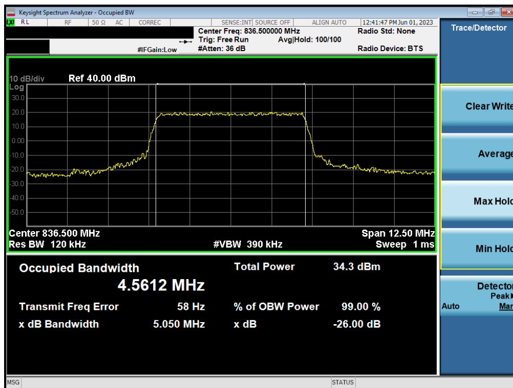
Plot 7-5. Occupied Bandwidth Plot (LTE Band 26/5 - 5MHz QPSK - Full RB Configuration)
