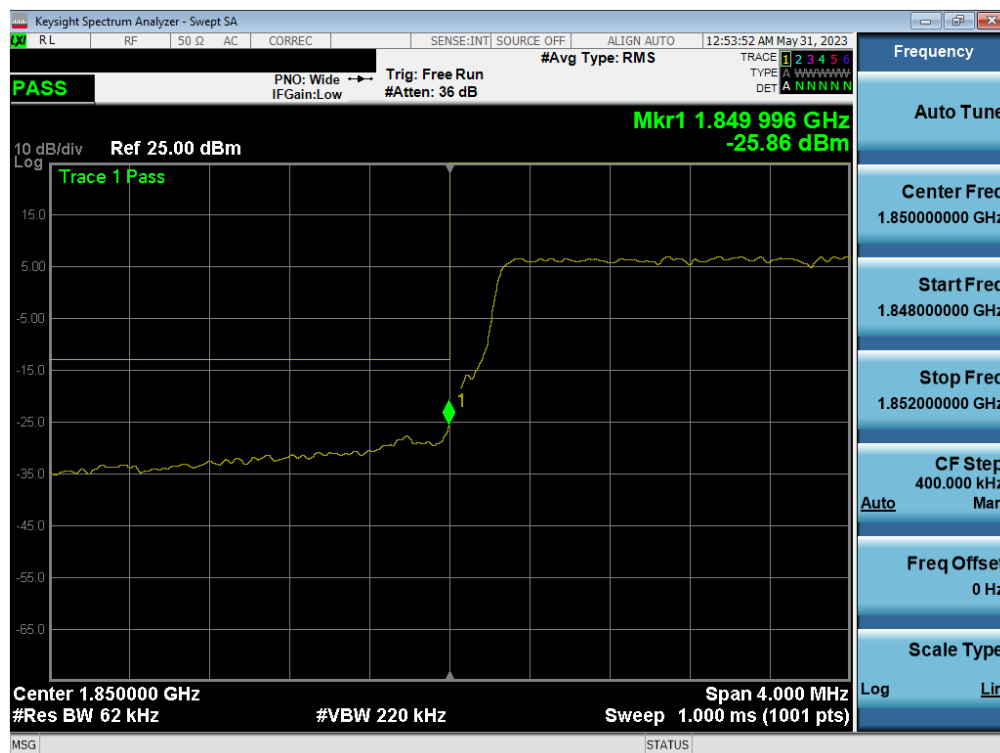
Plot 7-40. Lower Band Edge Plot (LTE Band 25 – 5MHz QPSK – Full RB Configuration)
