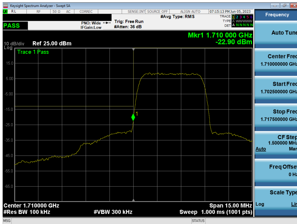
Plot 7-124. Lower Band Edge Plot (WCDMA AWS – Ch. 1312)
